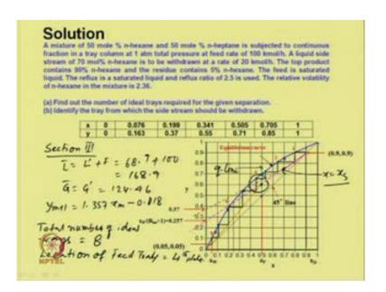
For section three, section three that is stripping section, the liquid flow rate L bar would be L dash plus F which is equal to 68.9 plus 100, which is 168.9; and gas rate is G bar would be G dash which is equal to 124.46, so the equations of the operating line for the stripping sections similar way we can write Y m plus one would-be equal to is coming out to be 1.357 x m minus 0.018.
