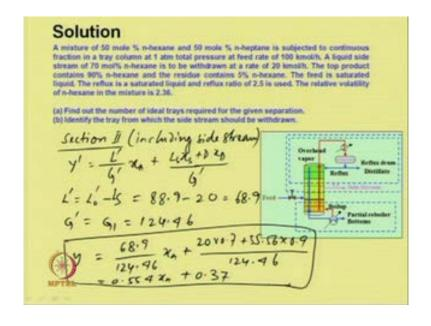
In this rectifying section, now section two, including side stream we have operating line equations, Y dash would be L dash by G dash into x n plus L s X s plus D x D by G dash, so we can write, L dash would be L naught minus L s, because the side stream is withdrawn, so the flow rate in this section would be reduced by L s, so it would be equal to 88.9 minus 20, which is equal to 68.9.
