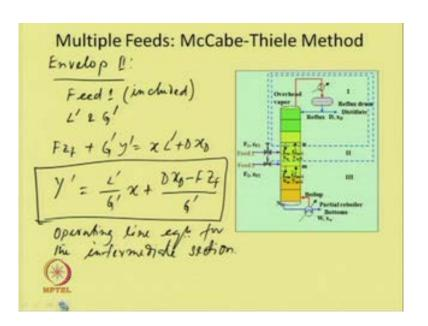
If we consider envelop two, it incorporates the feed one. Then we can calculate L dash and G dash from the vapor and liquid compositions which is from the fluorides of the liquids and gas in each tray. Now, if we do the overall material balance, it would be F z F plus G dash y dash, it would be equal to x L dash plus D x D; so we can write, Y dash would be equal to L dash by G dash into x plus D x D minus F z F divided by G dash.
