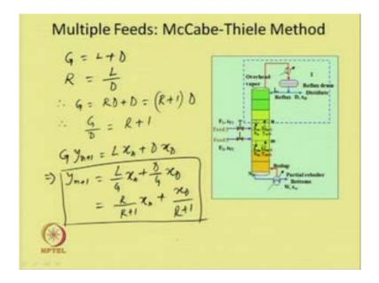
Let us see how to handle this problem, so we will do the material balance for each components and the mass balance. There are primarily three sections: section one above the feed tray, and then the second section which includes the feed one, and then stripping
