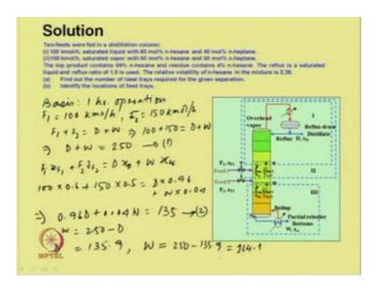
Let us take a basis of 1 hour operation. So F 1 is given 100 k mol per hour and F 2 is given which is 150 k mol per hour, if we do the total material balance then F 1 plus F 2 would be D plus W, which we can write 100 plus 150 would be equal to D plus W; we can write D plus W would be equal to 250, suppose this equation one.
