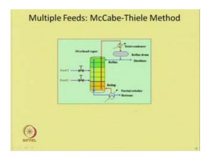
Let us consider multiple feed problems, and we can solve it similarly, like McCabe-Thiele methods. So, this is a distillation column where two feeds are introduced at two different trays, feed one and feed two should have the different compositions, and then two feeds we can handle in the same fractionators.
