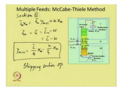
Now, we will consider the stripping section, as we did earlier, if we do the martial balance, it would be L n bar x n is equal to G m bar Y m plus 1 plus W X W; and if we put G m bar is equal to G bar is equal to L m bar minus W is equal to L bar minus W, then Y m plus 1 would be equal to L bar by G x m minus W by G bar X W. This is the equation of the operating line we have discussed earlier in the stripping section, operating line, and this is for section three.
