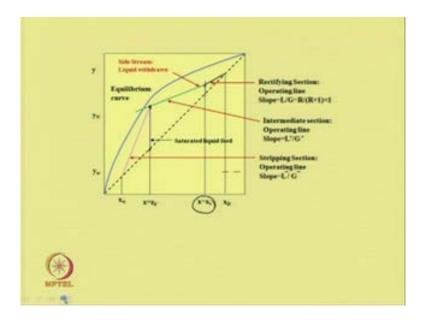
And, we can plot the operating line, this is the operating line for the stripping section, and this is operating line for the intermediate section, where it intersects at x is equal to x
