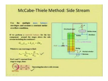
We can use the multiple mass balance envelopes, as we did before. First envelop we will consider without considering the side stream. So, we will get the operating line for the rectifying section, this is the operating line for the rectifying section.
