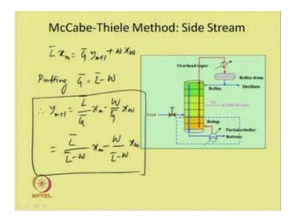
Now, if we do the material balance for the stripping section, L bar x m would be G bar y m plus 1 plus W X W, and if we rearrange this, we could write putting G bar would be L bar minus W. Therefore, we can write y m plus 1 would be L bar by G bar X m minus W by G bar x w, which is equal to L bar, L bar minus w x m minus W by L bar minus W X W, so this operating line equations for the stripping section.
