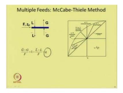
Suppose, this is the feed plate, and we know the feed flow rate and compositions, and then we can write the slope of the q line, which we discussed earlier; this is slope of q line, and which based on that you can see where the feed line will intersect.
