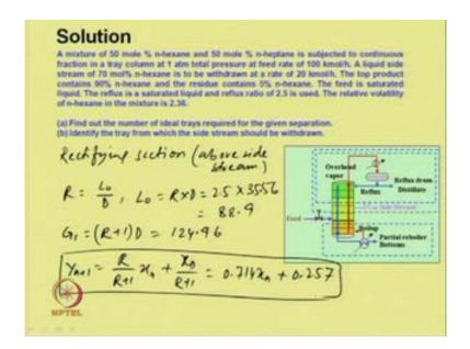
Now, let us consider the rectifying section, rectifying section above side stream, above side stream, R is equal to L naught by D, so L naught would be R into D which is equal to 2.5 into 35.56, and it should be 88.9; and G 1 would R plus 1 into D, and which is equal to 124.46. Now equations of the operating line, Y n plus 1 would be R by R plus 1 x n plus x D by R plus 1 which is equal to 0.714 x n plus 0.257, this is the equations of the operating line.
