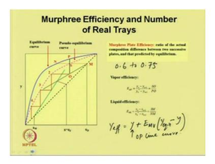
As we said the Murphree efficiency we can define as the ratio of the actual composition difference between the two successive plates and that predicted by equilibrium. So there are two types of Murphree efficiency we can define, one is in terms of the vapor, another in terms of the liquid.
