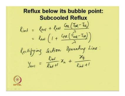
So we can write R internal would be equal to R external plus R external into CPR into TBR minus TCR divided by lambda. So, this we can write R external into 1 plus CPR, TBR minus TCR divided by lambda this term. So the rectifying sections operating line Y n plus 1 would be equal to R internal divided by R internal plus 1 x n plus x D divided by R internal plus 1.
