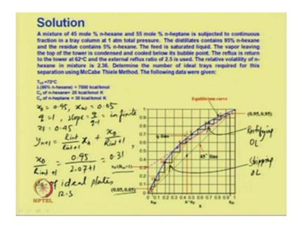
Now, the data which are given x D is 0.95 x W is 0.05, q is equal to 1 saturated liquid. So slope is equal to q by q minus 1 is equal to infinite. So this is the point, feed point and this is the q line which is vertical line at the feed point of 0.45 because z F is 0.45. So, we can calculate y n plus 1 would be R internal divided by R internal plus 1 x n plus x D by R internal plus 1. So, intersect x D by R internal plus 1 would be equal to 0.95 by 2.07 plus 1, which would be equal to 0.31.
