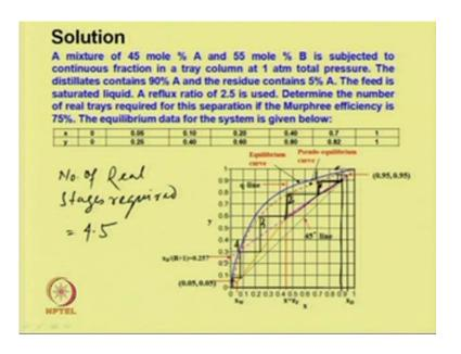
We plot from this line and if we plot the staircase construction from this point, so the number of stages would be one, two, three and this is four. Total number of real stages required is equal to 4.5. The staircase construction is drawn between the operating line and the pseudo equilibrium line which is drawn using the Murphree efficiency.
