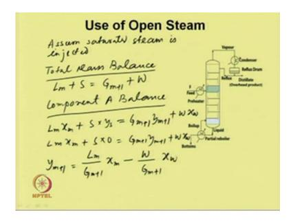
Now, we will do the total mass balance and material balance over the stripping section. We assume saturated steam is injected, then the total mass balance L m plus S is equal to G m plus 1 plus W and component balance, A balance if we do that we can write, L m X m plus S into Y S is equal to G m plus 1, y m plus 1 plus W XW. Now, if we solve it Lm X m plus S into 0 would be equal to Gm plus 1, y m plus 1 plus W XW. It will give Y m plus 1 would be L m by G m plus 1 X m minus W by G m plus 1 X W.
