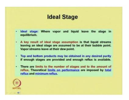
Now ideal stage; what is ideal stage, if the vapor and liquid leave a particular stage are in equilibrium then we call it equilibrium stage or ideal stage. A key parameters or important results for ideal stage assumption is that, the liquid streams leaving in a ideal stage are assumed to be at their bubble point and vapor streams leave at their dew point. This is the important assumptions for if we assume a stage is in ideal.
