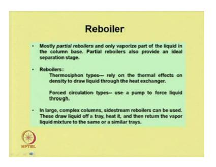
Now reboiler, most of the cases we use the partial reboiler; that means, only partially vaporized part of the liquid in the column base. So, partial reboiler also considered as an ideal stage or one extra stage. The reboilers are of different types; one is thermosiphon types, which rely on the thermal effects on density to draw liquid through the heat exchanger.
