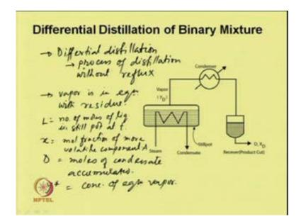
Let us consider differential distillation of a binary mixture. So, we will consider binary mixture a and b, and we will consider without reflux. When the batch distillation without reflux is operated, the process is called differential distillation. Since there is no reflux, the vapor which is producing from the still is assumed to be in equilibrium with that liquid, which is the residue; vapor is in equilibrium with residue.
