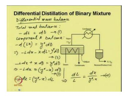
Now if we do the total material balance, the differential mass balance we will do. First, we will do the total material balance is minus dL is dD; say this is equation 1. Now component A balance we can write minus d of Lx would be equal to y star dD.
