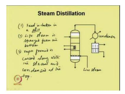
So, this is shown in the figure. As we can see, the feed is taken in a tank and live steam is injected through the sparger. Feed is taken in a still and then live steam is sparged from the bottom. So, the vapor which will produce it will carried by the steam and it is condensed. This is condenser. Vapor formed is carried along with the steam and condensed at the top.
