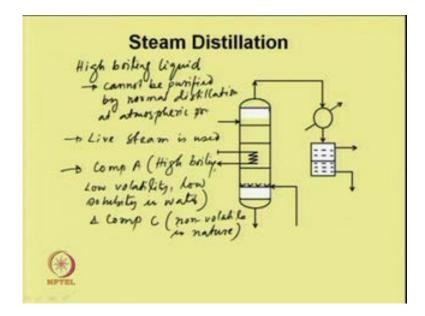
Let us consider another type of distillation which is steam distillation, particularly when some liquid which are very high boiling and it has some contaminant of non volatile components, which cannot be separated at normal distillation at atmospheric pressure. So, first is high boiling component. High boiling liquid cannot be purified by normal distillation at atmospheric pressure; because if we apply high temperature, there is a high possibility of decomposing the material at high temperature.
