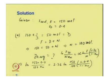
So, first we will try to calculate the average compositions of the distillate. It is given the feed, which is F is equal to 150 mol, and the composition Z F which is 0.4; 40 mol percent n-hexane, and for problem 1, it is given that to vaporize one-third of the feed. So, feed is vaporized one-third; that means 150 into one-third. So, 50 mol is vaporized which is D. From the total material balance if we look, F is equal to D plus W. So, 150 is equal to 50 plus W; so, the W is 100 mol.
