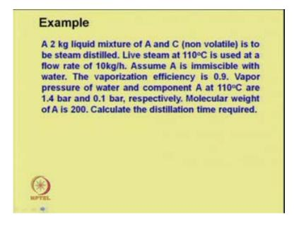
Now, let us take a very simple example. A 2 kg liquid mixture of A and C, which is non volatile is to be steam distilled. Live steam at 110 degree centigrade is used at a flow rate of 10 kg per hour. Assume A is immiscible with water. The vaporization efficiency is 0.9. Vapor pressure of water and component A at 110 degree centigrade are 1.4 bar and 0.1 bar respectively. Molecular weight of A is 200. Calculate the distillation time required.
