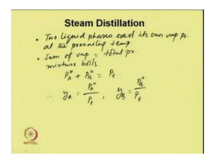
Now two liquid phases exert its own vapor pressure at the prevailing temperature, and this cannot be influenced by others. When the sum of the vapor pressure equals the total pressure, then the mixture boils. So, we can write P A v plus P B v is equal to P t. Therefore, y A should be P A v by P t; P A v and P B v are the vapor pressures of the components, and P t is the total pressure, y B should be P B v by P t. So, these are the vapor compositions.
