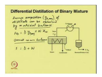
Now, the average composition y D average; so, this is y D. This can be obtained average composition, that is, y D average of accumulated distillate can be obtained by material balance. So, if we do the little balance F Z F is equal to D y D average plus W x w, and then we can do the overall mass balance, F is equal to D plus W. So, from this, we can calculate y D average.
