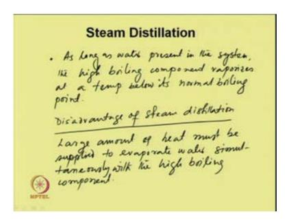
This means as long as water present in the system, the high boiling component vaporizes at a temperature below its normal boiling point. The disadvantage of the method: Large amount of heat must be supplied to evaporate water simultaneously with the high boiling component.
