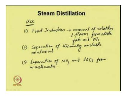
Now, what is the use of this steam distillation? Use importantly. This is used in food industries for the removal of volatile materials, volatiles, and flavors from edible fats and oils, separation of thermally unstable material and third, separation of ammonia and VOCs volatile organic materials from waste water, and so on. There are so many applications.
