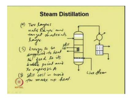
Now since, A has the less miscibility with water it will form two layers, and one layer is water layer and target materials layer. Then it is separated. This two layers can be easily
