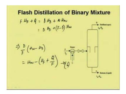
We can also write this plus this. Now, similarly if we use energy balance equation F H F plus Q is equal to D H D plus W H W. Now, if you substitute D H D plus F minus D H W and if we rearrange this equation in similar way, we can get D by F into H W minus H D would be equal to H W minus H F plus Q by F. This is equation 6.
