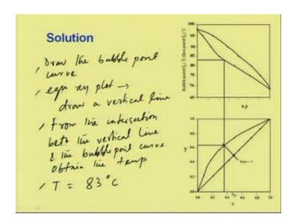
So, first we have to draw the bubble point curve curve and then the, from the equilibrium points equilibrium x y plot, draw a vertical line and then from the intersections between the, from the intersection section between the vertical line and the bubble point curve, obtain the temperature. So, the temperature is around in this case is around T is about 83 degree C.
