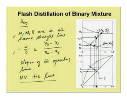
So, this points D which is H D and y D and here w which is H W x W, this point represent H W x W and the point which is given over here is H F plus Q y F and this is corresponding to x F, all these three points 1 2 and 3, say this is M and this is say W. So, W M D are in the same straight line and minus W by D and y D minus x F divided by x
