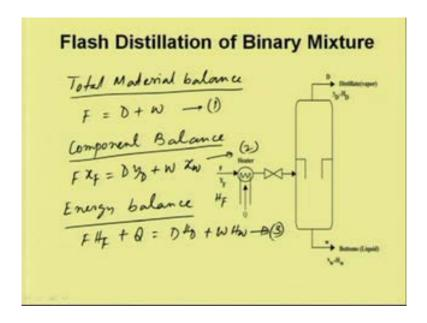
So, if you do the overall materiel balance, total materiel balance we can write F would be equal to D plus W, equation 1. If you do the component balance, balance for a we can write F x F is equal to D y D plus W x W. Similarly, we can write the energy balance equation, energy balance equation this is equation number 2. Energy balance equation should be F H F plus, this is H F plus Q would be equal to D H D plus W H W, this is equation 3.
