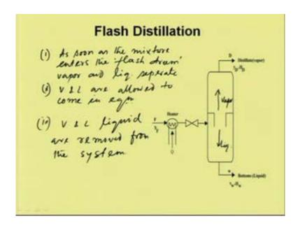
So, the vapor and liquid there, liquid goes down, vapor goes up. As soon as the mixture enters the flash drum, vapor and liquid separate. Then vapor and liquid are allowed to come in equilibrium, vapor and liquid are allowed to come in equilibrium. So, the enough space is provided and then finally, the vapor and liquid are removed from the system. This flash drum is very common particularly in petroleum industries, petroleum refining.
