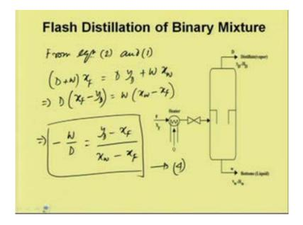
Now, from equation 2 and 1 we can write D plus W x F would be equal to D y D plus W x W. And from here we can write D into x F minus y D would be equal to W x W minus x F from which we can write minus W by D would be equal to y D minus x F divided by x W minus x F.
