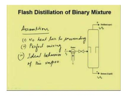
So, with this nomenclature if we do the materiel balance, first we will have the following assumptions. One is low heat loss to surrounding, perfect mixing and ideal behavior of the vapor, ideal behavior of the vapor. Now, let us do the steady state materiel balance on this flash drum.
