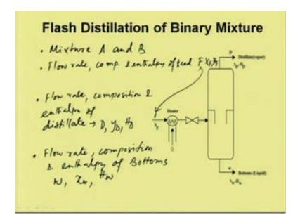
Now, we will consider a binary mixture in flash distillation and considered a mixture which contains A and B. Now, flow rate composition and enthalpy of feed, this is we can write F is the feed florid x F and h F, which is given over here. Then the flow rate composition and enthalpy of distillate which is given over here at the top, we can assume D y D y D and H D. The flow rate composition and enthalpy of bottoms, that is we can write W x W and H W.
