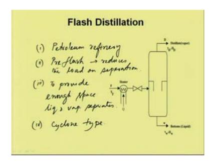
So, in many cases in distillation also they are sometimes we use the pre flash. So, it reduces the load on separation. So, in this designing of flash drum, it is very important to provide enough space, so that the liquid and vapor separates, liquid and vapor separates. In general the design of these sometimes it is of cyclone type.
