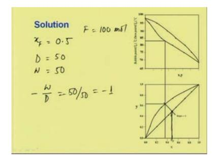
So, we have x F is 0.5 and D is 50 mol percent is vaporized, D is 50 mol if we assume feed F is 100 mol as the basis, then D is 50 mol and W is 50 mol. So, minus W by D would be minus 50 by 50. So, it would be minus 1. Now, this is the value at x F which is at 0.5 and then with the slope of minus 1, we will draw the line the equilibrium data which are obtained from the equations which is given y is equal to alpha x divided by 1 plus alpha minus 1 x.
