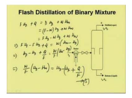
So, this is equation 4. Now, using equation 3 and 1, we can write F H F plus Q would be equal to D H D plus W H W, this is equation 3. Now, if you substitute D by F minus from the total materiel balance F minus W H D plus W H W and then we can write this
