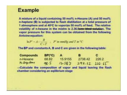
So, this is equation 9. Let us considered an example, a mixture of a liquid containing 50 mole percent n hexanes and 50 mole percent n heptanes is subjected to flash distillation at a total pressure of one atmosphere and at 40 degree centigrade to vaporize 50 mole percent of the feed. The relative volatility of n hexane in the mixture is 2.36, the vapor pressure for this system can be obtained from the following Antoine equations which this problem we have already discussed in our first lecture.
