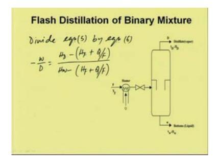
So, if we divide equation 5 by equation 6 we would obtain minus W by D would be H D minus H F plus Q by F divided by H W minus H F plus Q by F, if we look into the H x y diagram.
