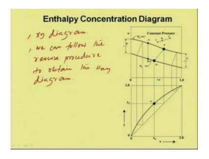
Similarly, if we have the equilibrium curve we can do in the reverse direction, we have the x y diagram then we can follow the reverse procedure to obtain the H x y diagram.
