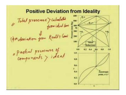
Now, we can see two types as we said one is minimum boiling Azeotropes, and another one is maximum boiling Azeotropes. Now, a mixture is total pressure - total pressure is greater than calculated from ideal law calculated from ideal law, then it shows the
