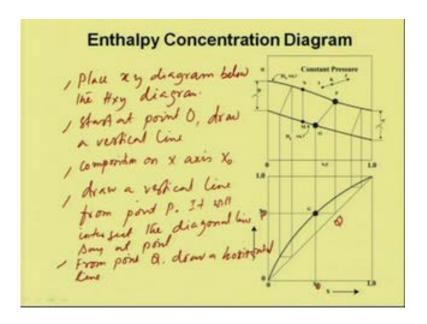
Now, let us see we have the equilibrium curve of H x y diagram, and point we will just place the x y diagram below the H x y diagram. Now, start at the liquid composition at
