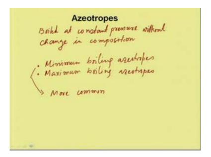
Azeotropes means it boils at constant pressure without change in composition, this is the azeotropic mixture. So, these Azeotropes have two different types; one is called minimum, minimum boiling Azeotropes, and second is maximum boiling Azeotropes; minimum boiling Azeotropes - this is more common.
