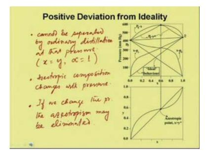
As we know at this composition a vapor composition will be same as the liquid composition, and it will boil at this constant temperature without change in composition. So, this type of mixture cannot be separated separated by ordinary distillation at that pressure.
