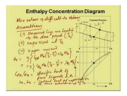
Now, it is very difficult to find out the mixture values, difficult to obtain if we assume we can get the approximate values assumptions, assume unmixed liquids mixed liquid are heated to the due points due points; that is T G, and second vaporized at T G and then
