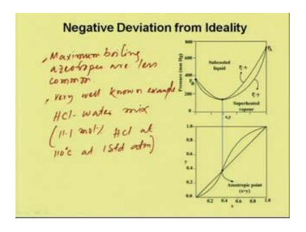
So, maximum boiling Azeotropes as we said before maximum boiling Azeotropes Azeotropes are less common, very well known examples known example are the Hcl water mixture at 11.1 mole percent Hcl at 110 degree centigrade temperature at one std atmosphere standard atmosphere pressure.
