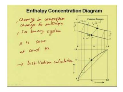
So, this is the typical enthalpy concentration diagram shown over here, and here as we know during distillation, during the change in phase, the change in compositions occurs change in composition, changes the enthalpy. So, this is the binary vapor liquid equilibria plots for binary system; it is plotted as enthalpy versus concentration at constant pressure, and this will be very much use full in distillation calculation.
