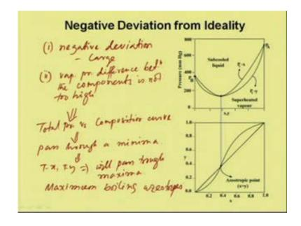
So, these are the Azeotropic point when negative deviation is large, negative deviation large and second is vapor pressure difference difference between the components is not too high. Then the total pressure curve total pressure pressure versus composition curve pass through a minimum, then the T x, T y curve will pass through a maximum. So, this is maximum boiling Azeotropes maximum boiling Azeotropes.
