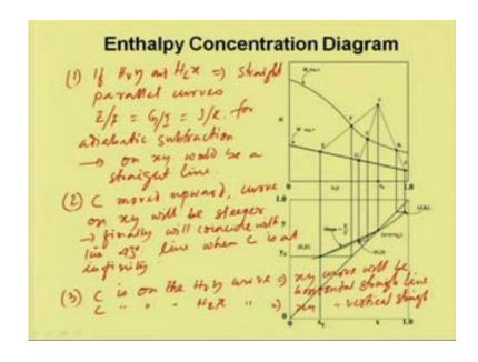
Three important observations, we can see one is if H v y and H L x, these curves are straight lines, straight parallel curves, then the ratio E by F would be equal to G by I would be equal to J by K for adiabatic subtraction. Then the corresponding curve on x y would be a straight line.
