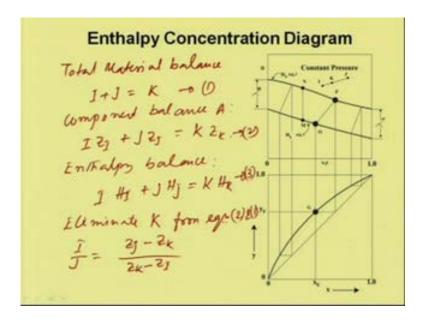
Now, if we do the material balance total material balance I plus J would be equal to K equation one, then the component balance component A balance, so I Z I plus J Z J would be equal to K Z k enthalpy balance I, this is two - I H I plus J H J is equal to K H
