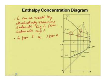
So, consider C can be result by adiabatically removing saturated liquid liquid; that is at point E from saturated vapor F and which is shown over here. This can also be considered removing adiabatically saturated liquid from G to G from I G from I or J from K, and any such combinations can be drawn and we can obtain C.
