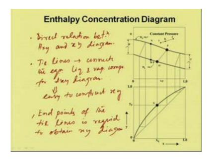
So, if we have enthalpy concentration relationship, we can have direct relation relation between H x y and x y diagrams, now if we have tie lines which connects connects the equilibrium liquid and vapor composition for H x y diagram, then it will be easy to construct x y diagram. So, only the end points of the tie lines end points of the tie lines is required to obtain x y diagram.
