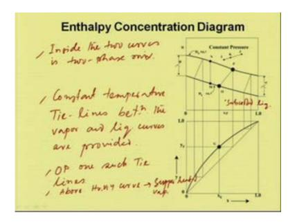
Now, inside this two curves inside this naval of is a two phase mixture, inside the two curves two curves is two phase mixture, and sometimes between these two curves constant temperature tie lines temperature, constant temperature tie lines between the vapor and liquid curves are provided O and P one such tie lines O P one such tie lines.
