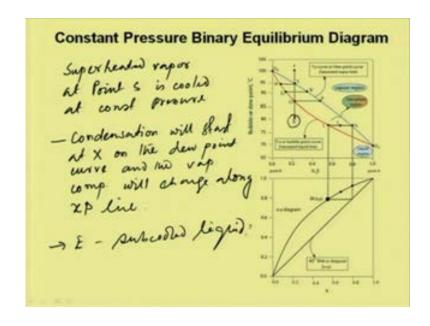
Now, if some amount of super heated vapor say at point S super heated vapor at point S is cooled at constant pressure what will happen? It will follow the same path in the reverse directions for examples condensation condensation will start at X on the dew point curve and the vapor composition will change along x P line. So, when the inter vapor is condensed and then liquid is again cooled so it will reach the domain at E which is sub cooled.
