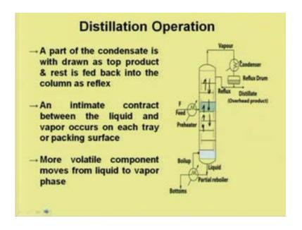
A part of the condense heat from this reflux dram is recycled back at the top and rest is taken as the product. So, the liquid fall down or flow towards down and there is intimate contact between the vapor and the liquid on each tray. So, more volatile component moves from liquid in this process the more volatile component from the liquid phase to the transfer to the vapor phase.
