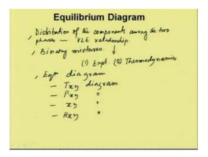
So, now the distillation process which is an equilibrium stage operation process it requires the vapor liquid equilibrium and physicochemical properties of the systems to solve this equilibrium stage operation. The distribution of the two components is governed by the vapor liquid equilibrium relationship, distribution of the components among the phases depends on the VLE vapor liquid equilibrium relationship.
