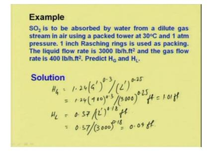
So, if we write these equations H G is equal to 1.24 G dash to the power 0.3 divided by L dash to the power 0.25 which is equal to 1.24, G dash is 400 pound per hour feet square to the power 0.3 divided by liquid flow rate is 3000 is to the power 0.25, this much feet. So, it is equal to 1.01 feet. H L which is 0.37 divided by L dash to the power 0.18 feet.
