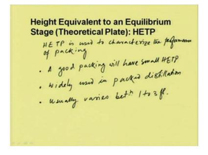
This HETP is generally used to characterize the performance of packing, HETP is used to characterize the performance of packing. So, the a good packing will have small HETP. This is widely used in packed distillation and its usually varies between 1 to 3 feet.
