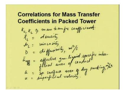
So, here k c and k L which is the mass transfer coefficients, rho L is the density, mu L is the viscosity, D is the diffusivity meter square per second, a effective is the effective gas liquid specific inter facial area of contact and a is the specific surface area of dry
