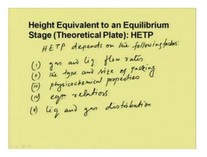
This HETP depends on the following factors, one is the gas and liquid flow rates, second the type and size of packing, physicochemical properties, the equilibrium relations and the liquid and gas distribution.
