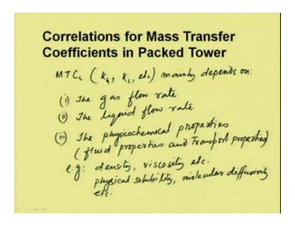
The mass transfer coefficients generally k G, small k G, k L etcetera mainly depends on the gas flow rate, second the liquid flow rate and third the physicochemical properties that is fluid properties and transport properties. So, the fluid proprieties like for example, density, viscosity etcetera and the transport properties like physical solubility, molecular diffusivity etcetera.
