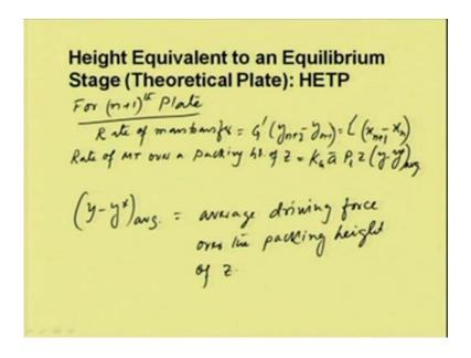
Then if we do the mass balance over n plus oneth tray for n plus oneth plate. So, rate of mass transfer is equal to G dash y n plus 2 minus y n minus 1 would be equal to L dash x n plus 1 minus x n. And rate of mass transfer over a packing height, height of z would be equal to k G a bar p t z into y minus y star average, where y minus y star average is equal to average driving force over the packing height of z.
