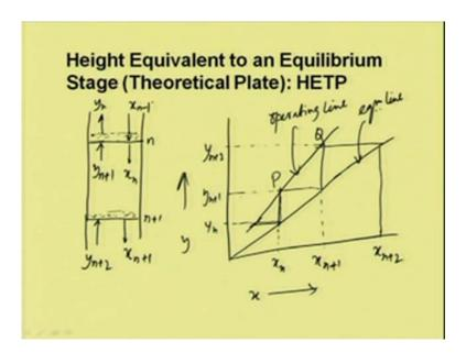
So, between this, this is operating line. So, between this point P and Q, it is reasonable to take the log mean overall driving force for y minus y star average.
