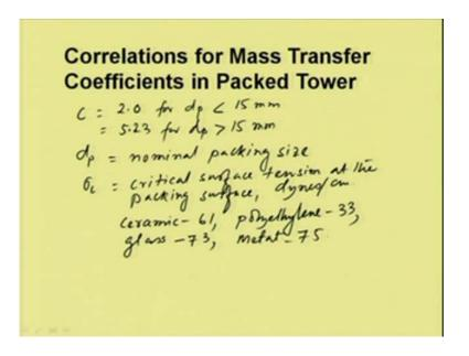
So, here this c, c is equal to 2.0 for d p less than 15 millimeter and this equal to 5.23 for d p greater than 15 millimeter, d p is the nominal packing size, sigma c is the critical surface tension at the packing surface in dynes per centimeter and it varies like for ceramic it is 61, polyethylene 33, glass 73 and metal 75.
