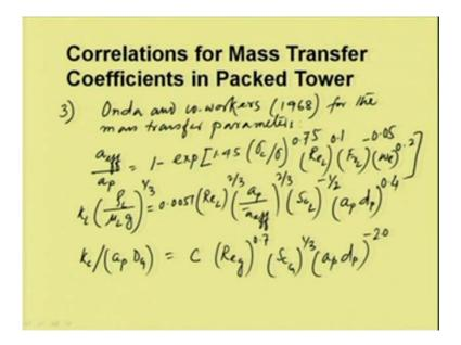
So, another correlation which is given by Onda and co-workers in 1968 for the mass transfer parameters, a effective divided by a p is equal to 1 minus exponential 1.45 sigma
