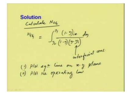
Now, we will calculate N t G; N t G we know that it is equal to integral y 2 to y 1 into 1 minus y i M divided by 1 minus y into y minus y i into dy. Now, we have to evaluate this integral, then to evaluate this integral we need to know the interfacial concentration; interfacial concentration, as we followed earlier we will follow similar procedure - first we will plot the equilibrium line, plot equilibrium line on x y plane, and then plot the operating line.
