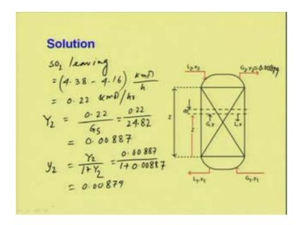
Then S o 2 which is absorbed is equal to 4.38 into 0.95 is equal to 4.16 k mol per hour. So, this is the amount absorbed, so the amount leaving from the tower. SO 2 leaving is
