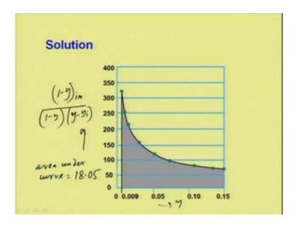
If we plot this versus y, this is basically 1 minus y i M divided by 1 minus y into y y minus y i. So, this is in this axis, and this is in this is y. So, if we plot this, then it will give the value area under the curve, which is N t G. So, area under the curve under the curve is equal to 18.05.
