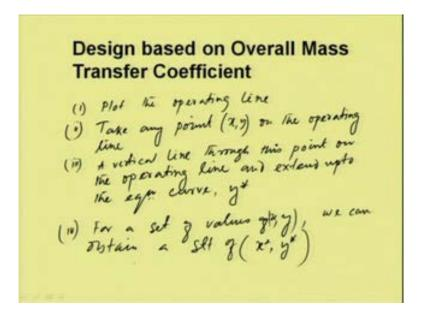
So far graphical integration we can follow the procedure, first plot the operating line, and then take any point x, y on the operating line, then we can draw a vertical line through this, through this point on the operating line, and extend up to the equilibrium curve curve which meets at a point y star. For a set of values of x, y we can obtain a set of set of x star y star, and then we can obtain the value of the integration.
