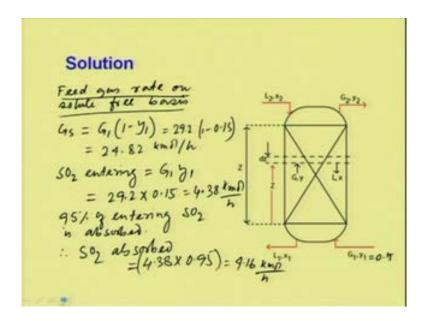
Now the feed gas rate on solute free basis, we can calculate feed gas rate on solute free basis. So, that is G s is equal to G 1 into 1 minus y 1 which is equal to 29.2 into 1 minus 0.15 which will give 24.82 K mol per hour, and the entering SO 2 is equal to G 1 y 1 which is equal to 29.2 into point y 1 is 0.15. So, 1 5 which is 4.38 K mol per hour, now 95 percent of entering entering sulfur dioxide is absorbed absorbed.
