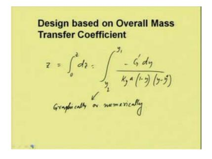
Now, the required packed height, we can obtain by integration of this equation. So, z would be equal to integral 0 to z dz would be integral y 2 to y 1 G dash dy by capital K y a 1 minus y y minus y star. So, now this integration can be done either graphically or numerically.
