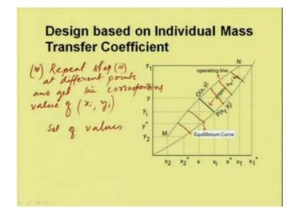
Now we can repeat this step and we can plot parallel to this line so many points on this curve, so repeat step three at different points and get the corresponding values of (x i ,y i) so then we have a set of set of values.
