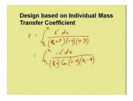
You can use other type of individual mass transfer coefficient to calculate the values of z, which is equal to we can write integral y 2 to y 1 G dash d y divided by K G a p capital K G into 1 minus y into y minus y i or we can also use integral x 2 to x 1 minus L dash d x divided by K L a capital K L a into C a average into 1 minus x into x i minus x.
