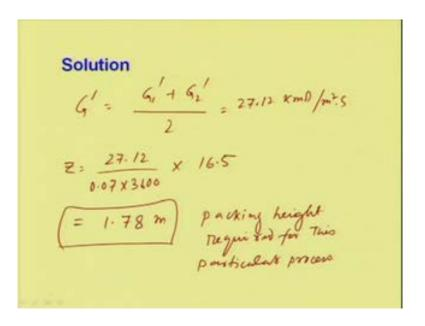
Now, we can get G dash which is G 1 dash plus G 2 dash divided by 2, which is equal to 27.12 k mol per meter square second. Now Z is equal to 27.12 divided by 0.07 into 3600 into 16.5, so this is equal to 1.78 meter. So this is the packed height required for this particular operation, particular process.
