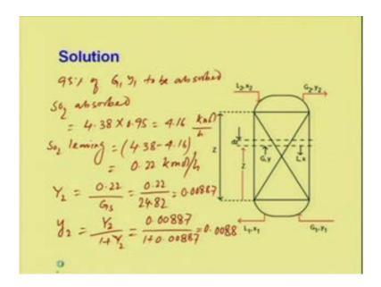
95 percent of G 1 y 1 to be observed, so then SO 2 absorbed should be 4.38 into 0.95 is equal to 4.16 k mol per hour. Now SO 2 leaving is equal to 4.38 minus 4.16 which is equal to 0.22 k mol per hour. Now, we can calculate concentration capital Y 2 is equal to 0.22 by G s which is 0.22 by 24.82 which is equal to 0.00887 and Y 2 we can calculate capital Y 2 by 1 plus Y 2 which is equal to 0.00887 divided by 1 plus 0.00887 which is equals to 0.0088.
