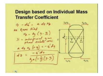
So from this we can write minus d G dash will be a d z into N A. Now we know that N A is equal to k y into y minus y i y where y i is the interfacial concentration, interfacial gas plate solute concentration. So if we put this in this equation the equation and then rearrange then it will be a d z N A into 1 minus y is equal to minus G dash d y, so d z equal to minus G dash d y divided by k y a into 1 minus y into y minus y i, so this is the equations for d z.
