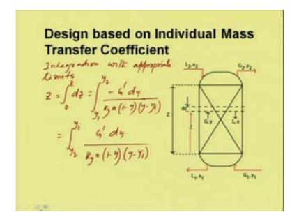
And then if we integrate this equation with the appropriate limits it gives z is equal to integral 0 to 2 d z will be equal to integral y 1 to y 2 minus G dash d y divided by k y a into 1 minus y into y minus y i is equal to integral y 2 to y 1 G dash d y divided by k y a into 1 minus y into y minus y i. Now, this evaluation of this integral will give you the value of z and this can be done by graphical or numerical methods.
