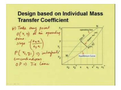
Now we will take any point on the operating line say at point O which is (x, y) take any point o x y on the operating line, now we know the slope of the value minus k x a by k y a, with this slope we can draw a line which is this line and which intersect at some point P which is (x i, y i) this give the interfacial concentrations corresponding to that (x, y) value, this line o p is called the tie line.
