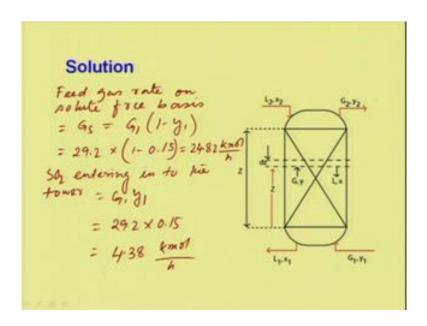
Now the feed gas rate on solute free basis we can calculate, solute free basis is equal to G s which is equal to G 1 into 1 minus y 1 which we can write 29.2 into 1 minus 0.15, so this will be 24.82 k mol per hour. Now SO 2 entering into the tower is equal to G 1 y 1 which is equal to 29.2 into 0.15 this is equals 4.38 k mol per hour. This is the entering sulphur di oxide concentration into the tower.
