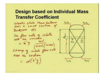
Now if we consider steady state operations of the column and if we consider the thickness at any point inside the tower is d z and a steady state mass balance over a small section of thickness d z will get the flow rate of solute with the carrier is equal to G dash y mol per time into area. Now the change of solute flow rate over the section change of solute flow rate over the section would be d into G dash y.
