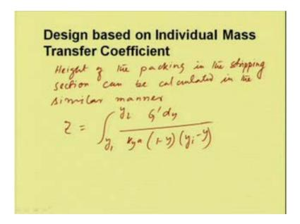
The height of the stripping section in the similar way, height of the packing in the stripping section can be calculated in the similar manner. So, the design equations we can write will be integral y 1 to y 2 G dash d y divided by k y a into 1 minus y into y i minus y.
