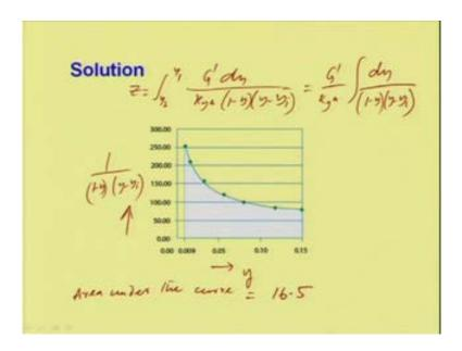
Now with that we know the equation which is z is equal to integral y 2 to y 1 G dash d y divided by K y a 1 minus y into y minus y i which is equal to we can write G dash by K y a integral d y by 1 minus y into y minus y i, so this area under the curve if we plot 1 by 1 minus y into y minus y i versus y then the area under this curve is equal to 16.5.
