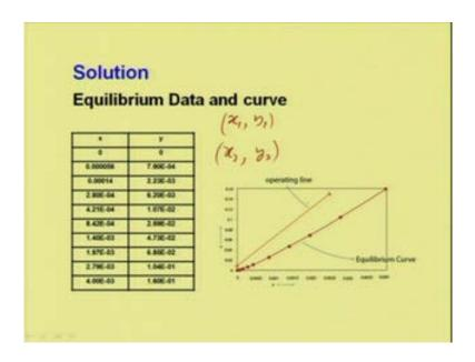
Now the equilibrium data which is given is plotted over here, we know the (x 1, y 1) and (x 2, y 2). With the equilibrium data given we can plot this is the equilibrium curve and with the data of (x 1 y 1) and (x 2 y 2) we can plot the operating line curve.
