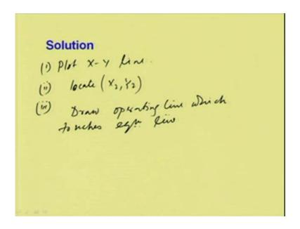
Now, what are the steps we follow, we plot the equilibrium line and then we locate x 2, y 2 and then we draw operating line. Line which touches equilibrium line and then point of tangency correspond to the minimum liquid rate.
