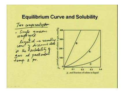
So, let us consider two component system, that means we will take a single gaseous component in contact with the liquid and the resulting concentration of dissolve solute, solute is the solubility of gas at particular temperature and pressure. So, suppose at a
