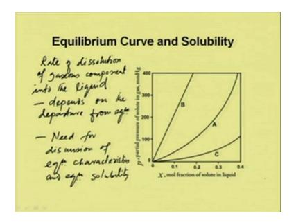
So, rate of the dissolution of gaseous component into the liquid depends on the departure from equilibrium. So, it is necessary to discuss the equilibrium characteristics and the equilibrium solubility of the gaseous components into the liquid. So, need for discussion of equilibrium characteristics and equilibrium solubility.
