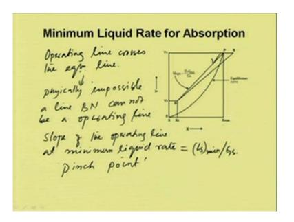
Now, in another figure we can see if we further reduce the liquid rate the operating line crosses the equilibrium line, that means in one section of the column absorption is taking place and in other section of the column desorption occurs, which is physically impossible. So, a line like BN cannot be a operating line. So, the operating line equation
