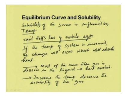
The solubility of the gases is influenced by temperature and it is follows Vant Hoffs law of mobile equilibrium. That means if the temperature of a system is increased, the changes will occur which will absorb heat. In most of the cases when gas is dissolved into the liquid then heat is evolved. That means if we increase the temperature which will decrease the solubility of the gaseous component. So, increase the temperature, decrease the solubility of the gas.
