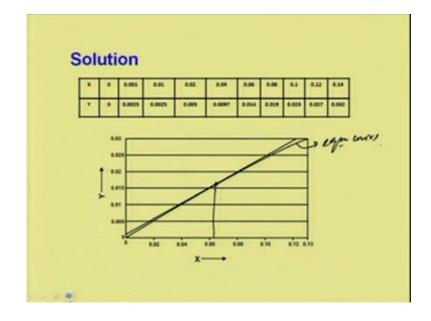
Then if we take the x y as the equation is given. So, this is the equilibrium data and this is the equilibrium curve and we know the point at the bottom of the tower and then we plot with the slope and it touches at this point.
