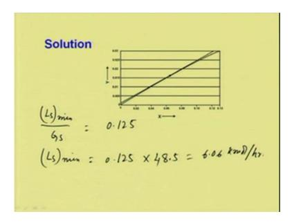
So, from this we can calculate L s min by G s, which is around 0.125 from the figure. So, L s minimum will be 0.125 multiplied by 48.5, so which is about 6.06 k mole per hour.
