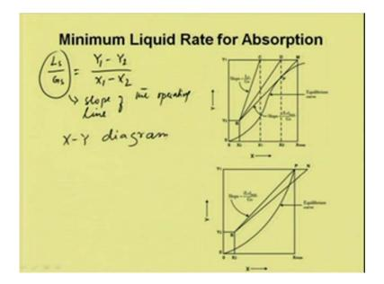
From these equations, we can write L s by G s is equal to Y 1 minus Y 2 divided by X 1 minus X 2. So, this is the slope of the operating line. Now, we know the terminal points Y 2 X 2 and we know the slope of the operating line and we can plot these operating line curve and which will cut the point Y 2 Y 1 line so that we can obtain X 1. So, this is the X Y diagram. So, there are two types of diagrams can be seen in which this is the equilibrium line and this is another equilibrium line.
