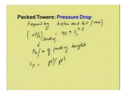
So, we can calculate the pressure drop for the packed towers and there is a correlation proposed by kister and Gill in 1991. That correlations can be used; delta P by L at
