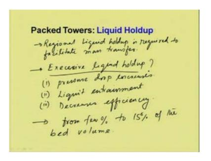
If there is excessive liquid holdup, what happens? The pressure drop increases; and there is a possibility of liquid entrainment; and third one is decreases efficiency. Generally the liquid holdup its permissible limit is around from few percent to 15 percent of the bed volume.
