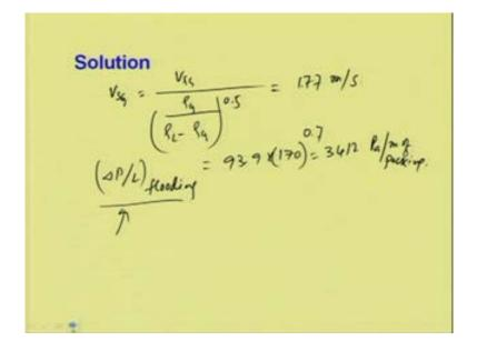
So now, we can calculate, V s G is equal to v f s divided by rho G by rho L minus rho G to the power 0.5 and substituting these values this is 1.77 meter per second. So, delta P by L flood, at flooding, the pressure drop we can calculate 93.9 into F p is 170 to the power 0.7 which is 3412 Pascal per meter of packing.
