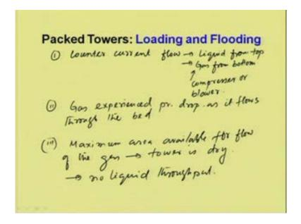
If we consider counter current flow in the packed towers; counter current flow liquid from top and gas from bottom liquid flows due to gravity and gas flows due to compression or the blower power, compressor or blower. Then when the gas flows and the liquid also flows from top to down; the gas experience pressure drop as it flows through the bed the maximum area available for flow of the gas when the tower is dry; that means, there is no liquid throughout.
