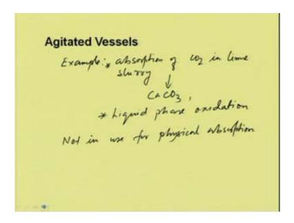
The agitated vessels are generally used for the gases which undergo chemical reactions with the liquid. And particularly for example for example, absorption of carbon dioxide
