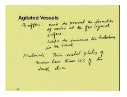
The baffles are generally used, baffles used to prevent the formation of vortex at the free liquid surface, and it also helps to increase the turbulence in the tank; and, the materials, generally, for the baffles, we can use thin metal plates of thickness less than 10 percent of the tank dia can be used as the baffles; generally 4 to 6 baffles are usually used for the agitated vessels.
