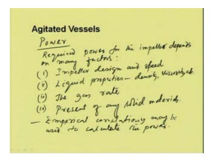
The power, the required power for the impeller depends on, on many factors. One of them is impeller design and speed, liquid properties such as density, viscosity, etcetera, the gas rate, or if any suspended solids are present, any solid materials. So, to calculate the power, there are several empirical correlations are available. Correlations may be used to calculate the power.
