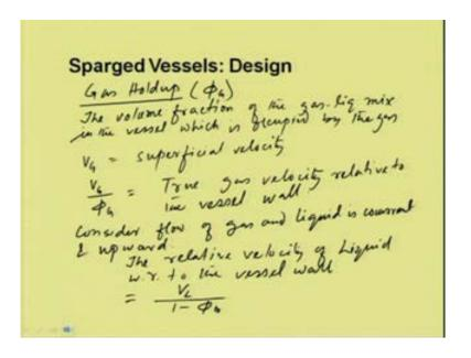
Now, the gas holdup we can calculate. The gas holdup is defined as the volume fraction, volume fraction of the gas liquid mixture in the vessel which is occupied by the gas. So, this is called as gas holdup and is defined as phi G and if we consider V G as the superficial velocity, then we can write, V G by phi G is the true gas velocity relative to the vessel wall. Now, if we consider flow of gas and liquid is cocurrent and upward, then
