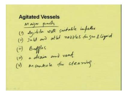
So, the major part for this agitated vessels are agitator with suitable impeller, inlet and outlet nozzles for gas and liquid, baffles, a drain and vent, manhole for cleaning. So, these are the major parts in mechanically agitated contactors. The impellers are available in different designs.
