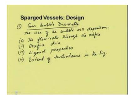
So, now, we will just see how to design the sparger. Through the sparger, the gas is generally bubbled. So, bubble size will change as it flows from bottom to top of the column. So, one is bubble diameter. The size of the bubble will depend on the flow rate through the orifice; second is the orifice dia, liquid properties and the extent of turbulence in the liquid. So, these are the major factors on which the size of the bubble will depend.
