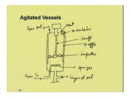
So, let us discuss, first, the simple equipment for gas dispersed, which is agitated vessels. The schematic of the agitated vessels, we can draw, sorry. So, this is a simple vessel, which is fitted with impellers. So, this is the stirrer shaft and this is vessel, installed with
