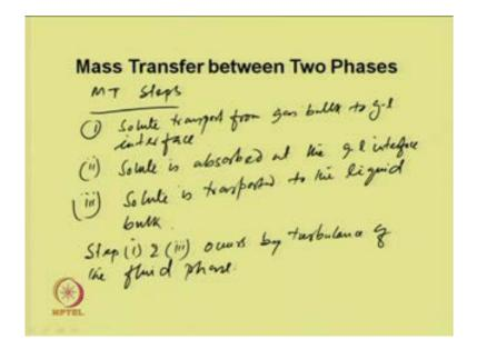
The concentration near the interface changes, and the mass transfer takes place in three steps; solute transport from gas bulk, to gas liquid interface, then at the interface, solute is absorbed at the gas liquid interface, and third solute is transported to the liquid bulk. The transfer of step one and three occurs by turbulence of the fluid phase.
