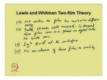
Third one; they said mass transfer within the film by molecular diffusion only. Bulk phases well mixed, so beyond these films, concentration in a phase is equal to the bulk concentration. Equilibrium exists at the interface. No evidence of these films in reality.
