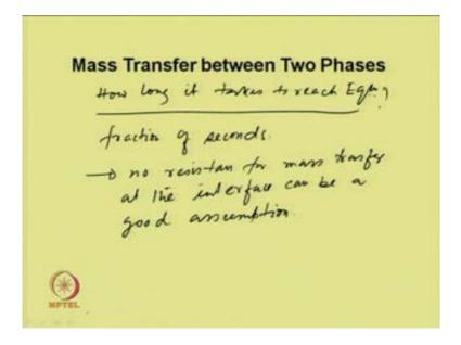
If the two phases are not in equilibrium, then how long it takes to reach equilibrium. To attain the equilibrium, it takes fraction of seconds. So, we called, there is no resistance at the interface for mass transfer at the interface, can be a good assumption.
