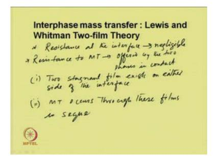
However, there are some exceptions in this case as well. As we said resistance at the interface is negligible, and resistance to mass transfer, offered by the two phases in contact. This is how the Lewis and Whitman in 1924, they visualized the interface mass
