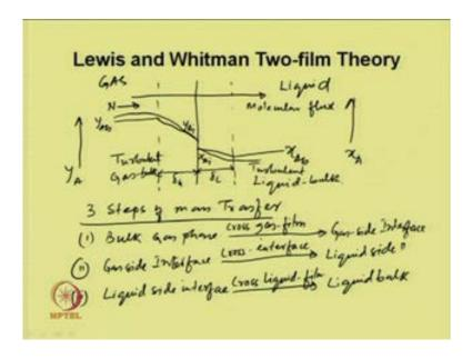
So, according this Lewis and Whitman two film theory, we can see that there is a liquid side film, and this is gas side film. This is a delta g and this is a delta l, liquid film, and
