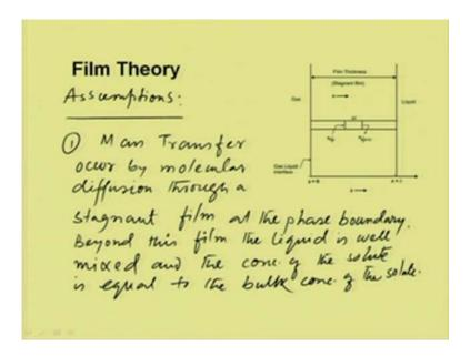
So, this theory, are based on certain assumptions. One is, mass transfer occur by molecular diffusion through a stagnant film at the phase boundary; that is, this one. Beyond this film, film, the liquid is well mixed and the concentration of the solute is equal to the bulk concentration of the solute.
