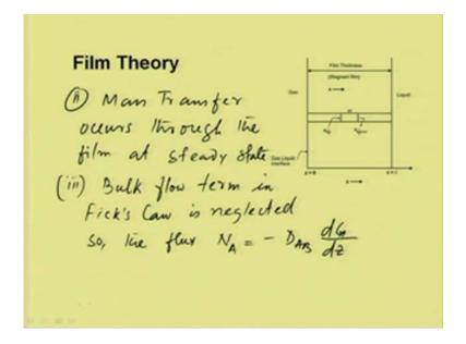
The second assumptions for this case, mass transfer occurs through the film at steady state. And third one is, bulk flow term in Fick's Law is neglected, neglected. So, the flux can be represented as is equal to minus D A B d C A d z.
