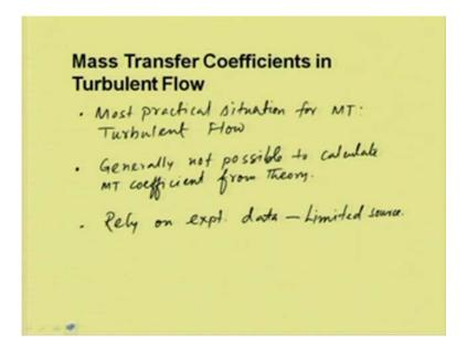
So now, we will start mass transfer coefficient in turbulent flow. In turbulent flow is the most practical situation for mass transfer, most practical situation is the turbulent flow. And, for turbulent flow, it is generally, not possible to calculate, generally, not possible to calculate mass transfer coefficient from theory. So, we have to rely on experimental data and these experimental data are of limited source.
