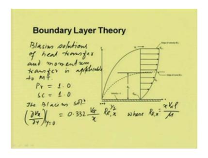
Blasius solution, solutions of heat transfer and momentum transfer is applicable to mass transfer. So, if we apply, for heat transfer, this solution is applicable when Prandtl number equal to 1. So, in this case, when Schmidt number for mass transfer is equal to 1, this is also applicable. For momentum transfer, the Blasius solutions can be written as del V x del y at y is equal to 0 is 0.332 V infinity by x Reynolds number x to the power half, where Re x is equal to x V infinity rho by mu.
