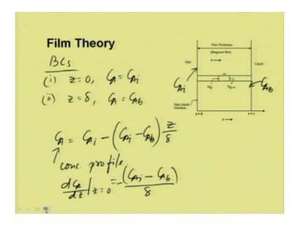
So, what are the boundary conditions, in this case? The first boundary conditions at z equal to 0, C A, we said, at the gas liquid interface C A i; So, C A will be C A i; and the second, at z equal to delta C A will be C A B; so, at the surface, so, C A B. So, if we integrate the equations, it will be C A, will be C A i minus C A i minus C A B z by delta. So, this is the concentration profile.
