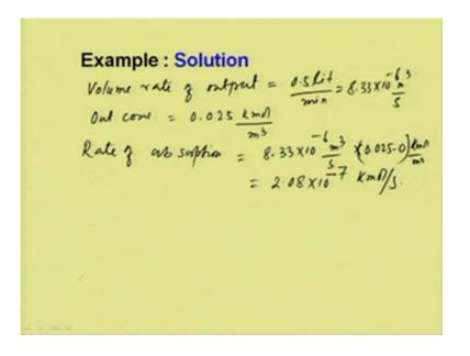
Now, we know, the volume rate of output, volume rate of output is equal to 0.5 litre per minute, which is equal to 8.33 into 10 to the power minus 6 meter cube per second. Now, the outlet concentration is given, is equal to 0.025 k mole per meter cube and we can calculate, the rate of absorption will be equal to 8.33 into 10 to the power minus 6 meter cube per second into 0.025 minus 0 k mole per meter cube, is equal to 2.08 into 10 to the power minus 7 k mol per second.
