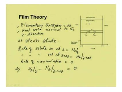
Now, let us consider a control element delta z, elementary thickness delta z and unit area, normal to the z direction, that is, the direction of mass transfer. So, at steady state, we can write rate of solute in, in at position z is equal to N A z; rate of solute out at z plus delta z is equal to N A at z plus delta z and rate of accumulation is equal to 0, at steady state. So, we can write the balance equations in N A at z minus N A at z plus delta z is equal to 0.
