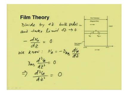
Now, if you divide this by delta z in both sides, and take limit delta z tends to 0; so, we will get minus d N A d z equal to 0. And, we know that, N A, as per the assumption, N A will be minus D A B d C A d z. So, substituting these values, it will be D A B d 2 C A d z 2 will be equal to 0. So, from this, we can write d 2 C A d z 2 is equal to 0. Now, if we integrate these equations with the boundary conditions...
