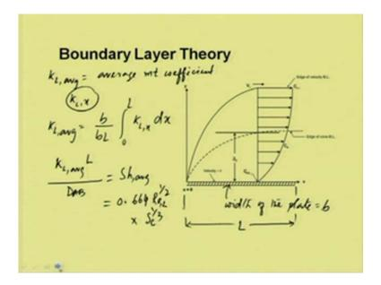
Now, the average mass transfer coefficients we can obtain K L average, we can obtain by integration of the equations of K L x with the, with the boundary conditions 0 to 1. So, K L average will be equal to B by, B is width of the plate, by B L; so, the length is L; so, B L integral 0 to L K L x D x. So, the result is K L average into L divided by D A B is equal to Sherwood number average is equal to 0.664 Re L to the power half into Schmidt number to the power one-third.
