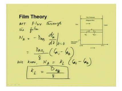
Now, at steady state, the mass transfer flux through the film is equal to N A minus D A B into d C A d z at z equal to 0. So, if we calculate d C A d z at z equal to 0 is equal to minus C A i minus C A B by delta. So, it will be D A B by delta C A i minus C A B, and we know that, N A will be K L C A i minus C A B. So, K L is equal to D A B by delta. So, this is the mass transfer coefficient which is directly proportional to diffusivity and inversely proportional to the film thickness.
