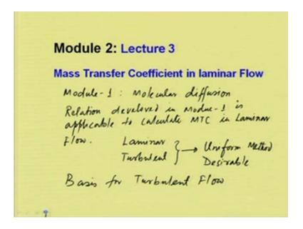
In module 1, we have discussed molecular diffusion and the relation developed in module 1 is applicable to calculate mass transfer coefficient in laminar flow. But a uniform method is desirable for the laminar and turbulent flow conditions; for laminar and turbulent, a uniform method is desirable. So, we will consider a simple case, and then, this lecture will make the basis for turbulent flow.
