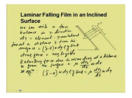
In this case, we can write a force balance in the y direction. Consider a element of fluid d y and the gravitational force acting on this element at distance z from the surface. So, we can write, this is, delta minus z w d y rho g sin theta; and, the drag force, if we considered negligible, then the retarding force due to viscous drag at z, at a distance z
