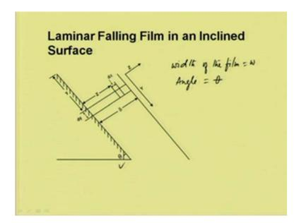
Now, let us consider another situation, where the laminar film is falling down a inclined surface. So, the depth of the liquid film is delta and width of the film is, is w, and the angle is theta.
