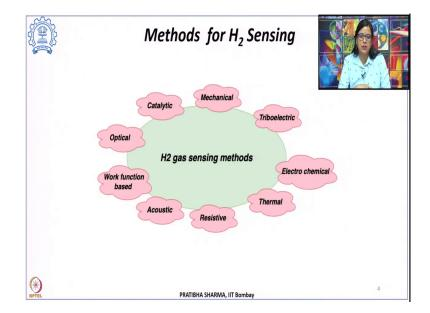
Now, based on the methods of hydrogen sensing, these can be classified into like mechanical sensors, triboelectric sensors, electrochemical sensors, thermal sensors, resistive sensors, acoustic sensors, work function based sensors, optical sensors and catalytic sensors. So, we will see very briefly these types of different sensors which can be used for hydrogen sensing.
