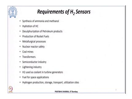
Like hydrogen sensors could be used during the synthesis of ammonia and methanol to identify any type of leak, hydrogen sensors are required at the process when the process is hydration of hydrocarbons or desulfurization of petroleum products, production of rocket fuels. For various metallurgical processes like galvanization or different types of other processes in the nuclear reactor safety.
