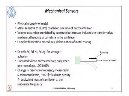
Now, the another class of sensors could be mechanical sensors and the sensing is done by the change in the physical property of the metal when it is subjected to hydrogen. For example, like if metal palladium is taken then palladium is actually coated on a micro cantilever.
