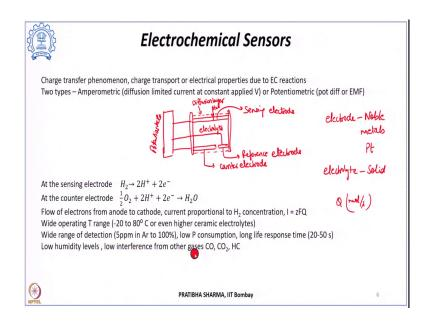
Now, the another type of sensor is electrochemical sensor. Now, these electrochemical sensors, they work on the principle of charge transfer phenomena. So, charge transfer taking place between the electrodes with an electrolytic medium. So, it is based on the charge transport or electrical properties which occurs due to the electrochemical reactions. So, these electrochemical sensors these are of two types, either amperometric sensors or potentiometric type.
