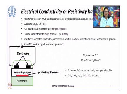
So, these are the general type of the electrochemical sensors which are used. Now, the another class of sensors is electrical conductivity or resistivity based sensor. So, as the name itself is suggesting, here in the electrical conductivity change or the resistivity change of the sensing element can be mapped to the hydrogen gas concentration. So, when there is a change in the resistance, that is measured as a reference for detection of the hydrogen gas.
