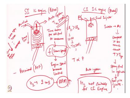
So, when we look into two aspects so, we have this spark ignition IC engine and then we have this compression ignition based IC engine. So, in spark ignition based typically petrol is conventional fuel that we used in compression ignition, diesel is the conventional fuel that is being used here.
