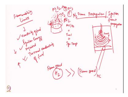
So, if you have any ignition source and you are giving a spark here. So, spark is given here and if there is a flame it will travel or it catches air or oxygen plus it follows fuel and plus it follows the ignition temperatures. So, ignition temperature will be there if this flame goes and transfers the heat to the nearby molecules of the fuel and oxidizer and there you will see that there is a flame front propagating.
