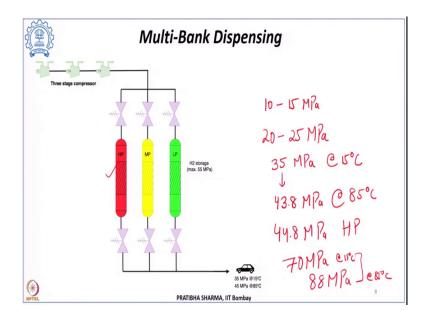
So, this was about the major components of the compressed and liquid hydrogen refuelling station there are different mechanisms through, which this filling can be done and like one of the concept is a multi bank dispensing. Now, in multi bank dispensing there are multiple storage banks like, there are three storage bank in this figure like a low pressure bank, a medium pressure bank and a high pressure bank.
