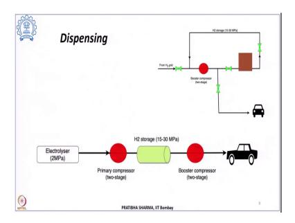
Now, the another possibility could be wherein when the hydrogen, which is let us say on site produced using an electrolyzer it is compressed and stored into hydrogen storage vessel, which is present at the hydrogen refuelling station and this is stored at a pressure between say 15 to 30 MPa that is, lower than the pressure that is desired for filling onto the car tank.
