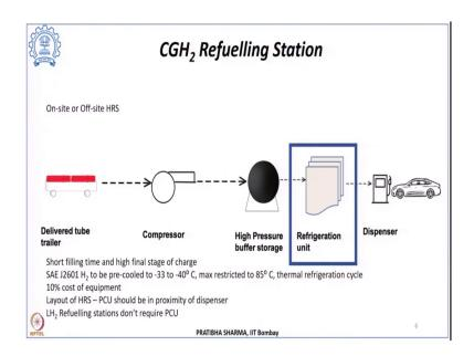
Now the, another important component which is in the compressed gas refuelling station is the refrigeration unit. Now, this is very important in the sense that we require a very short fueling time when a car arrives at a refuelling station we want that it should be fueled in a minimum time with a least waiting time and the filling should be at the maximum allowable.
