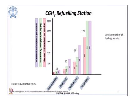
Now, depending upon what is the capacity of this buffer storage there can be different types of hydrogen refuelling station. Now the future hydrogen refuelling station has been categorized into either very small hydrogen refuelling station, small, medium or large hydrogen refuelling station. Depending upon what is the maximum hydrogen throughput per day in kgs, what is the average hydrogen throughput per day and the number of cars that arrive approximately per station?
