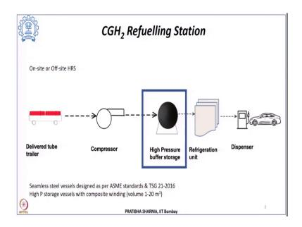
Now, in a typical compressed gas hydrogen refuelling station the hydrogen which is carried from the distribution terminal through delivery tube trailers this is at a certain pressure that we have seen in the last class. It is compressed using a compressor from the tube trailer pressure to the high pressure buffer storage pressure.
