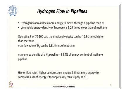
Now, when we consider hydrogen flow in pipelines, we know that it takes more energy to flow hydrogen as compared to natural gas through a pipeline. So, it is roughly around 4 times more energy to move hydrogen in a pipeline. We also know that the volumetric energy density for hydrogen is 3.29 times lower than that of methane.
