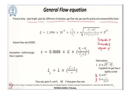
And that has been created using pipe length, pipe diameter, difference of elevations, gas flow rate, gas specific gravity and the compressibility factor. Now there are other equations that can also be used like the pan handle A, pan handle B or it could be Weymouth equation, all these can be used also for finding the pressure drop or flow rate.
