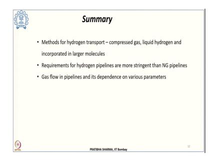
To summarize in this class, we have seen the different methods of hydrogen transport that could be used like the transport in the form of compressed gas as liquid hydrogen and it can also be incorporated into larger molecules transported over long distances as liquids. We have seen specifically the transport of hydrogen in hydrogen pipelines and the requirements for hydrogen pipelines these are more stringent than the natural gas pipelines.
