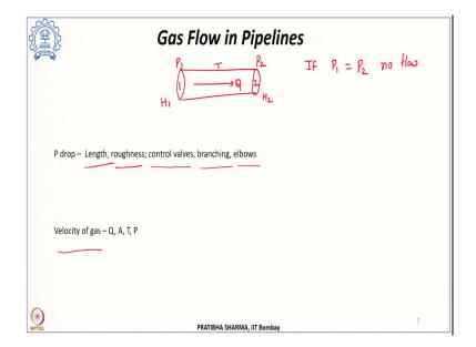
Such that the inlet pressure is  $P_1$ , outlet pressure is  $P_2$ , the elevation of point 1 is H1 that of point 2 is H2, the flow is Q, it is held at a temperature T. Now if we consider the flow inside a gas flow in a pipeline, we know that the flow of gas in a pipeline is because of pressure difference. If the two pressures are same then there will not be any flow of gas inside the pipeline.
