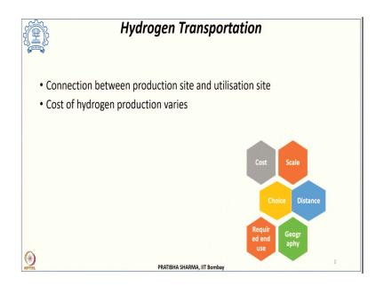
Now connecting the point of hydrogen production with the point of utilization is very much essential and their hydrogen transportation plays a major role. Now the low density of hydrogen that is the biggest bottleneck and that makes the hydrogen transportation very expensive. The options to tackle with this challenge is we can either compress we can either liquefy or we can incorporate hydrogen into larger molecules all these methods we have already studied.
