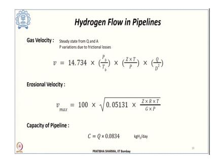
Another characteristic that needs to be considered is the gas velocity. If we consider the flow to be steady state in that case it can be derived from either like the volume flow rate and the area of cross section at a given temperature and pressure; however, since during considering the flow inside a pipeline, the pressure variations which arises because of the frictional losses, this velocity also changes and that velocity can be given by this particular relationship.
