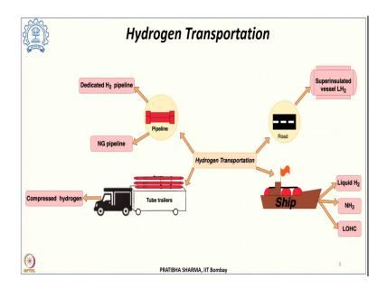
Now for that either it can be carried in the form of compressed hydrogen through road by means, of tube trailers or it can be carried through pipelines. So, either we can use the existing natural gas pipelines for hydrogen transport or we can have new infrastructure with dedicated hydrogen pipelines or it can be taken over long distances in larger scale through ships as liquid hydrogen or it can be carried in form of liquid hydrogen through road using super insulated vessels.
