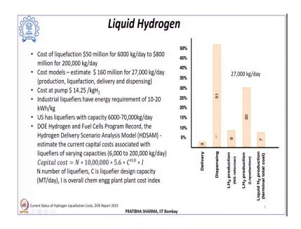
Now, the another option for storage is in the liquid form. Now, the cost of liquefaction depending upon the capacity like if it is 6000 kg per day or if it is 2,00,000 kg per day the cost could be in the range of 50 million dollars to 800 million dollars and there has been several studies which has been carried out. There have been different cost models including all the production, liquefaction, delivery and dispensing cost being included to and that has estimated that.
