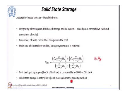
Now, when absorption-based systems like the metal hydride-based storage systems are being considered. It is found that these are at par with the compressed hydrogen tank. So, there has been studies carried out where in integrating electrolyzer with a metal hydride-based hydrogen storage system and fuel-cell system it is found that these are currently at par they are already cost competitive with the 700 bar compressed hydrogen tanks.
