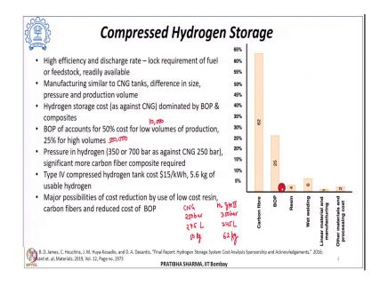
So, depending upon the requirement of fuel and feedstock, we can achieve the required efficiency and discharge rate. At the same time, these can be readily available wherever it is required. Now, the compressed hydrogen tanks they are manufactured in the same manner as the compressed natural gas tanks, like we use type IV tanks where these are made up of inner liner and with a completely wrapped fiber resin composite.
