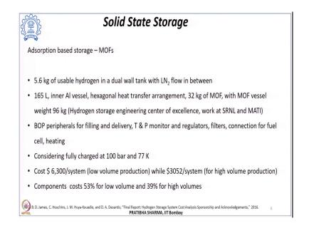
Now, if we consider the adsorption-based storage say for example, with metal organic frameworks, these systems are made up of because we have learnt that adsorption materials, they store hydrogen at liquid nitrogen temperatures.
