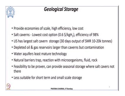
Now, when it comes to geological storage, the natural gas storage in the geological structures has been well proven and it has been widely used, this particular method of storage that provides economies of scale. It has high efficiency, low cost, it has low land cost lower footprint requirement above ground. And then we have also seen that there are different ways or geological structures in which we can store hydrogen like it can be in salt caverns.
