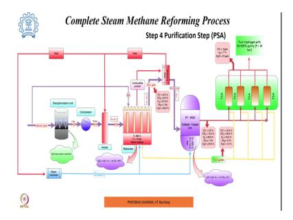
In the last step which we have seen today is purification step, finally, the product gas obtained after water gas shift goes to the pressure swing adsorption unit, wherein there is a batch process; however, using multiple adsorbent bends beds can made it continuous. And after PSA we get pure hydrogen with a purity of 99.999 percent pure at a pressure of approximately 14 bar.
