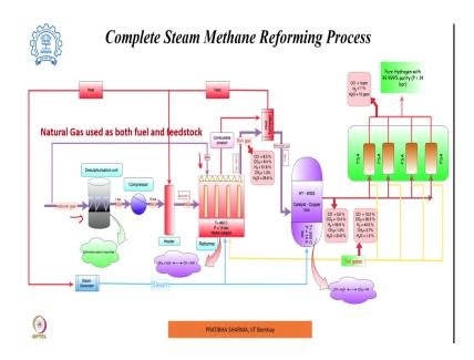
Now, let us see them together, so that we can know about the complete steam methane reforming process. Now, as we have seen natural gas acts as both fuel and feedstock in the steam methane reforming process. So, it acts as a feedstock entering into the desulphurisation unit and it acts as a fuel and supplies the required heat to the burners of the steam methane reformer.
