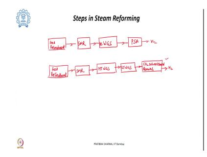
Now, today we will see the 4th step in the steam reforming. So, the last step which is the purification step that determines which water gas shift reaction reactor will be there. If it is pressure swing adsorption is the purification technique which is being utilized then only high temperature water gas shift reactor will be there.
