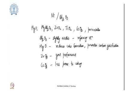
So, these are ideally the requirements when a catalyst support is being looked at. For industrial scale hydrogen production mostly nickel on alumina support is being used as a catalyst in the reformer tubes. Other than alumina there are several other catalyst support which are being studied like magnesium oxide, magnesium aluminium oxide, zirconia, titania, ceria these are the other support which are being studied and reported in the literature.
