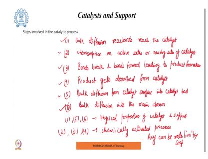
We know that when we are talking about a catalytic process, in the catalytic process on the surface of the catalyst the reactants adsorb, they undergo different reactions, bonds are formed, bonds are broken and finally, the product is formed and then catalyst returns back to its original initial state.
