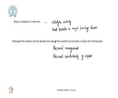
Now, we have seen that there are challenges associated with the reformer and the major limitation in the reformer seems that the catalytic activity could be the major challenge, but it has been observed that the catalytic activity definitely could be the rate limiting step but at the same time the heat transfer characteristics, the heat transfer is prominently or the major limiting factor when it comes to the operation of a steam methane reformer.
