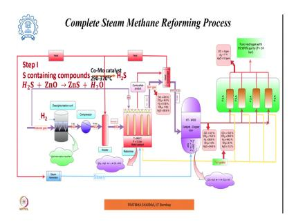
In the first step a small split steam of hydrogen from the product side is used for catalytic hydrogenation of sulphur containing compounds on a sulphur tolerant catalyst, which is
