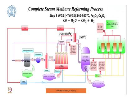
Now, the next step as we have seen is water gas shift reaction, wherein more hydrogen can be extracted. Carbon monoxide reacts with steam to produce carbon dioxide and one more mole of hydrogen. This reaction occurs at a temperature of 340 to 360 degree centigrade and this is slightly exothermic reaction; that means, it will be favored at lower temperature.
