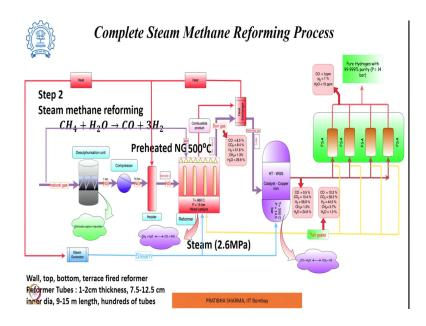
Now, these are tubular reformers tubular box type of furnace, wherein depending on where the burner is located these can be either top fired reformer, bottom fired reformer if the burners are on the bottom side, side fired reformer or terrace fired reformer.
