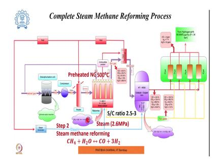
Now, once the sulphur containing impurities are removed in the desulphurisation unit, the treated natural gas goes to the second step which is the steam methane reforming process wherein methane is pretreated and the sulphur containing impurities are removed.
