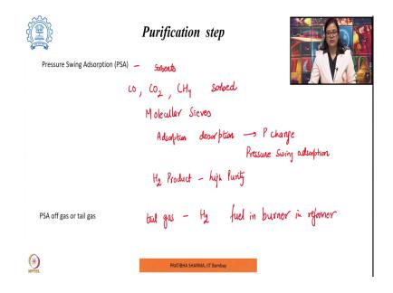
If however, pressure swing adsorption is used for purification in that case various adsorbents can be used. So, different sorbents can be used wherein on the surface of which the impurities like carbon monoxide, carbon dioxide, methane can get sorbed, so that we can remove all these impurities and we can get pure hydrogen as the product.
