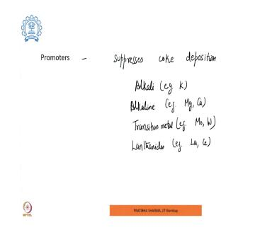
Now, other than the catalyst and support, a small quantity of promoters are added and this addition of promoters suppresses coke deposition onto the catalyst surface. The catalyst promoters are used includes alkali metal elements like potassium, alkaline magnesium and calcium. Transition metal based including molybdenum and tungsten from the lanthanide series, lanthanum and cerium.
