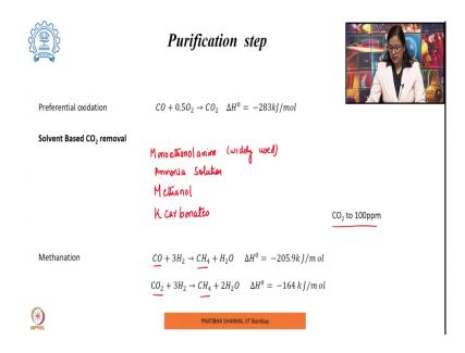
So, if solvent based carbon dioxide removal method is being used, in that case we know that from the low temperature water gas shift less than 1 percent of carbon monoxide is left and that can undergo preferential oxidation to convert into carbon dioxide.
