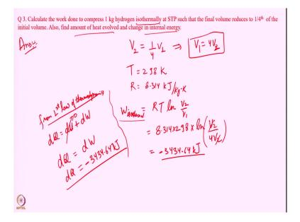
So, what is the amount of work that need to be done to compress 1 kg of hydrogen isothermally at standard temperature and pressure. Such that the final volume will reduce to one-fourth of the initial volume, we have to also find out the amount of heat evolved and change in internal energy. So, here it is given that the of such as the final volume reduces to one fourth of the initial volume.
