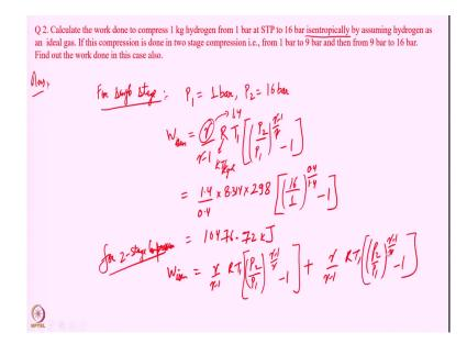
So, for doing the for doing a small calculation how the compression is being done, the question is we have to calculate the work done to compress 1 kg of hydrogen from 1 bar to 16 bar at standard temperature and pressure by assuming hydrogen as an ideal gas. If this compression, we will do in two stage compression that is initially we will go from 1 bar to 9 bar and then from 9 bar to 16 bar then we have to calculate the work done in this case also.
