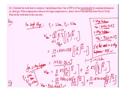
So, initially we have to compress it from 1 bar to 9 bar and then from 9 bar to 16 bar. So, in this case  $P_1$  is equal to 1 bar,  $P_2$  is equal to 9 bar and  $P_3$  is given by 16 bar. So, now after that we have to put the value of these, it is 1.4/0.4. Similarly, the R value is 8.314 T is 298, initially the P2 is we have to compress it from 1 bar to 9 bar; so, P2 is 9, gamma minus 1 is 0.4, 1.4 minus 1.
