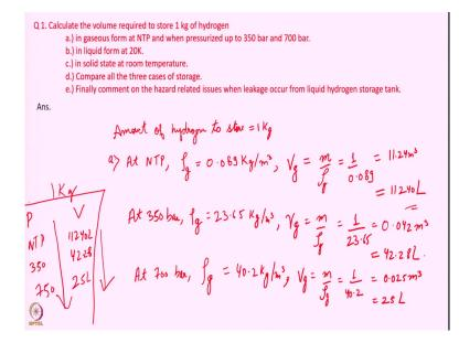
So, in the first question we have to calculate the volume required to store 1 kilograms of hydrogen. First, the first question is that it will how what amount of volume we require to store in gaseous form at normal temperature and pressure. And when you pressurize it up to 352 or bar to 700 bar; then we will store we will try to find out the volume when hydrogen will be stored in liquid form of 20 kelvin, in then in the solid state at room temperature.
