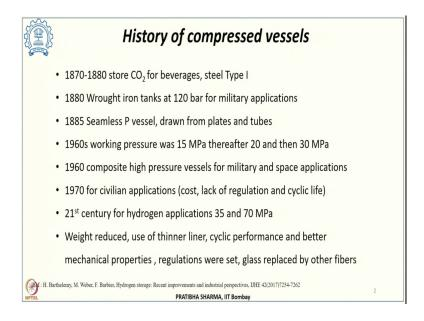
Thereafter, in 1880 hydrogen, it was stored at 120 bar in Wrought iron tanks and this was for military application. In 1885, the use of seamless pressure vessels which were in fact drawn
