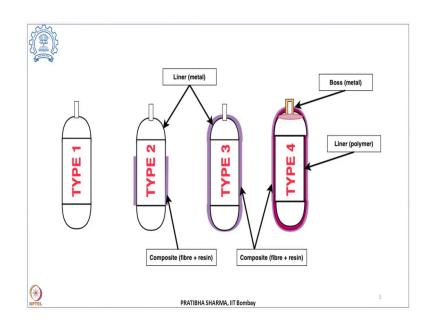
Just to show you how these tanks are. So, type I tank, this is a completely metallic tank with one port being shown here. This is all metal tank and this is highest in weight, but lowest in cost. Now, the type II tank, this is again a cylindrical structure with there could be 2 domes on the other side and only the hoop is wrapped. So, this is the hoop wrapped with the polymer reinforced; this is fiber and resin composite.
