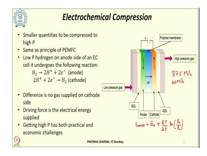
So, it has components like a PEMFC it has membrane electrode assembly where the two electrodes and membranes are integrated with electro catalyst to form an assembly MEA then there are gas diffusion layers, bipolar plates, current collectors and the end plates. The major difference of an electrochemical compressor from a polymer electrolyte membrane fuel cell is that gas is not passed on to the cathode side.
