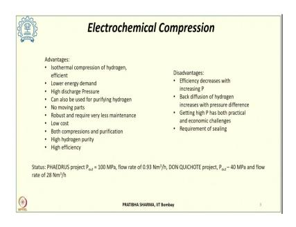
The reason being what happens is as we increase the pressure the Nernst voltage becomes almost of the same order of magnitude as that of the ohmic losses and as such the efficiency decreases. Secondly, if we further increase the pressure, in that case the permeation of hydrogen from the cathode side onto the anode side the process which is known as back diffusion will also increase.
