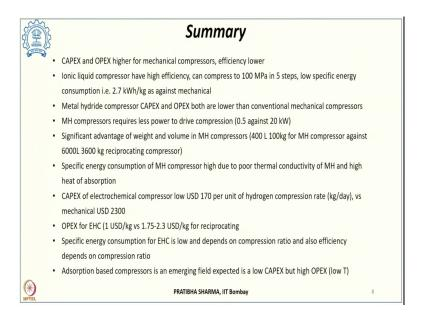
To summarize the CAPEX and OPEX is both higher for mechanical compressors they have many moving parts, maintenance cost is higher their efficiency is lower. We have seen the ionic liquid compressors which have high efficiency and we can achieve higher compressions higher pressures like 100 MPa in five steps, they require low specific energy like 2.7 kilowatt hour per kg and that is as against the mechanical which require high energy.
