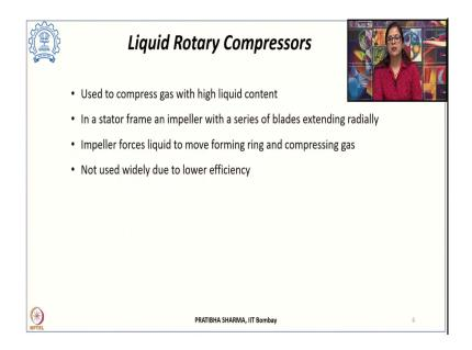
So, these type of compressors can; that was a liquid piston type of compressor, we can also have a liquid rotary type of compressor and these rotary type of compressors these are specifically used to compress gas which has a high liquid content. So, that is a saturated gas, which has a very high liquid content can be compressed using these liquid rotary type of compressors.
