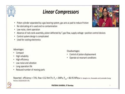
Now, in these type of compressors, the biggest advantage is that they have a sort of gas bearing system which separates the piston cylinder and this gas bearing system it also acts as a sort of that reduces the friction and losses. So, without even the using of the lubricating oil, we can reduce with the use of this gas bearing system which can act as a pad to reduce the friction.
