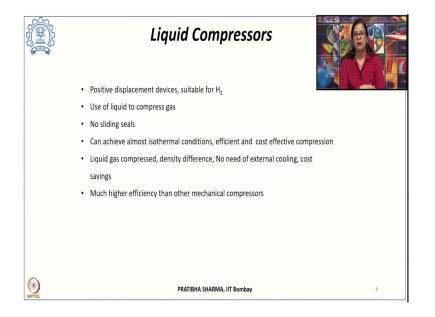
Now, the another class of compressors which can be used for hydrogen and they are very much suitable for hydrogen compressor are the liquid compressors. Again, they are the positive displacement type of devices and they compress hydrogen with the use of a piston, but that piston is now a liquid. So, the movement or the compression of the gas is provided by means of a liquid as such these are known as liquid compressors.
