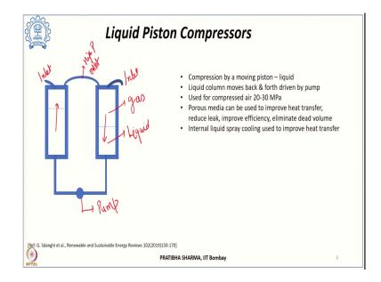
Now, if we look at these type of compressors, then we have two chambers which are connected by means of a pump which controls the flow, we have liquid and gas in these compression chambers which are connected by means of pump. And then we can have compression and expansion in these two chambers and there are inlet walls and then you can get a high pressure hydrogen at outlet.
