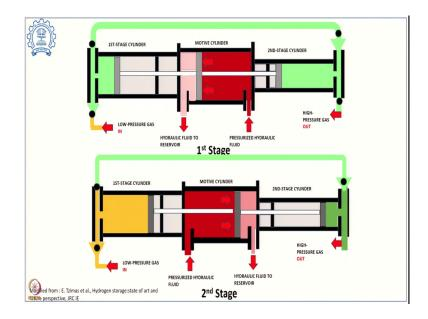
Now, to consider a two stage compression, for a reciprocating type of compressor, this figure shows the first figure shows the 1st stage of compression; the second figure shows the 2nd stage of compression. To explain the principle of operation in the beginning, a low pressure gas which is hydrogen in our case is taken in the first stage of compression. So, the first stage cylinder, this is having a higher diameter compared to the second stage cylinder.
