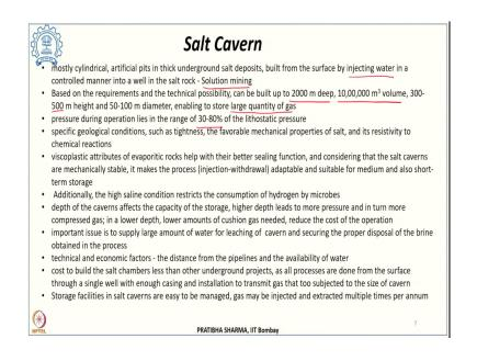
Now, let us first look at the salt cavern based storage. Now these salt cavern based storage these are usually the cylindrical type of structures and these are artificial pits which are formed in the thick underground salt deposits. And these are built from the surface and these are made by means of either injecting water in a controlled manner inside a well in the salt rock this is also known as solution mining method.
