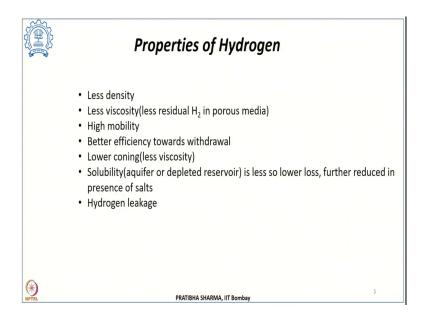
Now, before going into the details of such structures for hydrogen storage, we need to understand the properties of hydrogen. Actually, this most of the knowledge that we have about the underground hydrogen storage that comes from the experiences that we had from carbon dioxide storage or from natural gas storage. However, the properties of hydrogen, that differs from carbon dioxide as well as natural gas.
