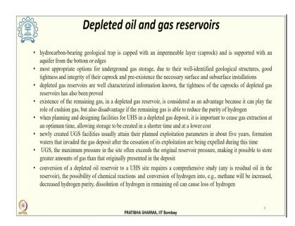
Now, the third option that can be used for storing hydrogen is depleted oil and gas reservoirs. Now these are hydrocarbon reservoirs which has a hydrocarbon bearing geological trap. So, there should be a trap which will be used for storing hydrogen and this has to be capped with an impermeable layer and that is known as caprock. This is actually supported by an aquifer which can be either present at the bottom of it or onto the edges.
