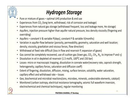
So, depending on that we can either have a pure hydrogen based storage or in the form of mixture of gases. So, whatever experiences which we are using in hydrogen storage in these structures that comes from either carbon dioxide storage where the carbon dioxide storage is basically meant for carbon dioxide sequestration which is long term phenomena which is a
