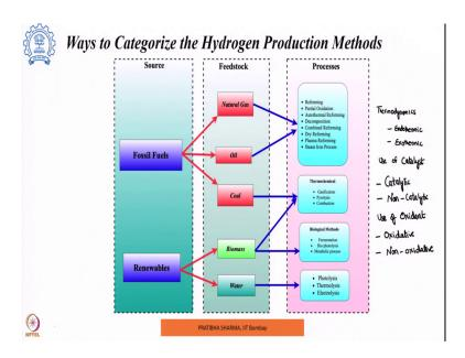
There are large number of ways for hydrogen production and there are different ways in which we can categorize these hydrogen production methods. For example, we can categorize them on the basis of the thermodynamics of the process; like, whether the processes which are used can be either endothermic or the process could be exothermic. We can categorize the processes of hydrogen production on the basis of use of catalyst, the process can be catalytic or it can be non catalytic process.
