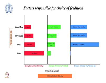
Now, if we look at these numbers, the theoretical amount of energy which is required to produce hydrogen from various fossil fuels as against from water by means of say electrolysis. The amount of energy which is required, theoretical amount of energy required per mole of hydrogen being produced is lowest if it is to be produced from natural gas. And the yield of hydrogen is high when it is being produced from natural gas as against compared to the other feedstock.
