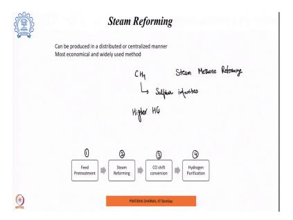
Now, let us start with the steam reforming process for hydrogen production. Now, this steam reforming as the name suggests steam is used as oxidant. This process can be either used in a distributed manner or a centralized manner. Distributed manner; where the requirement of hydrogen is small. At the same time if it is locally produced on site such that it can fuel the requirements of smaller end use applications or refueling station.
