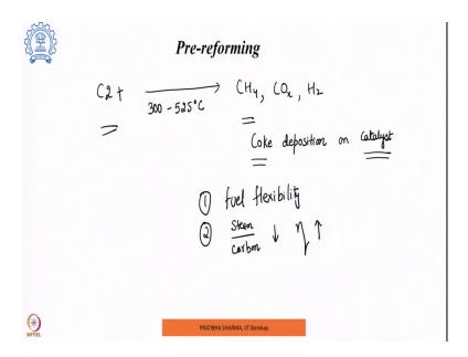
So, any of the C two plus hydrocarbons are being used in the reforming process then they have to undergo an additional step which is known as pre reforming step wherein these hydrocarbons are converted into lower hydrocarbons specifically methane carbon monoxide or carbon dioxide and hydrogen. So, this additional step is only in case of where the higher hydrocarbons are being used. Else in case of methane reforming this is not required.
