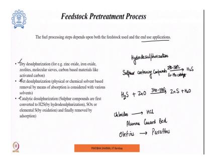
So, let us look at the first step which is the Feedstock Pretreatment Process herein it depends which feedstock is being used for hydrogen production. Say for example, if methane is being used for hydrogen production in that case the major impurities which we can see could be sulfur containing impurities which needs to be removed.
