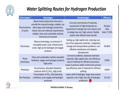
We can also get hydrogen, we have seen through various water splitting routes, either thermochemical route or electrolysis or photoelectrochemical or photolysis route. Now, the major problems associated with thermochemical cycles are corrosion and toxicity of the materials. Requirement of high temperatures, requirement of design of low cost reactor as well as low cost materials, high volume is required.
