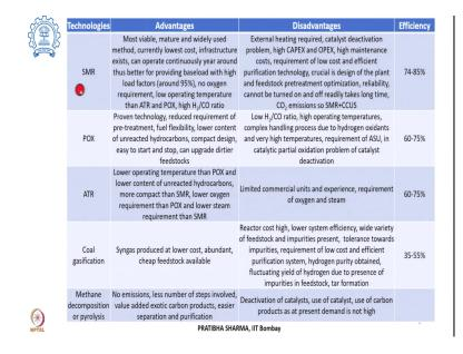
Now, when we compare the different technologies and see their advantages and disadvantages, the first technology which is most widely used one is the steam methane
