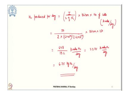
Now, to find out that much amount of hydrogen per day we can write it as this is current divided by the number of electron transfer, charge on the electron, Avogadro's number  $N_0$  and this will give us hydrogen produced in kilo moles per day.
