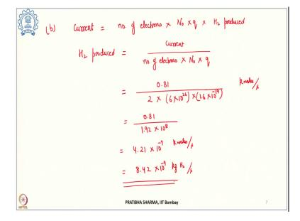
So, let us calculate that part, so in part b we have to calculate the amount of hydrogen being produced. Now we know that the current that flows through the spell is number of electrons
