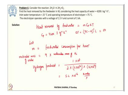
So, the last problem that we will do today is the reaction for water splitting into hydrogen and oxygen is given in which takes place in the electrolyzer. It is considered that the feed water is used to remove the heat and the amount of heat which is removed we have to find out by the
