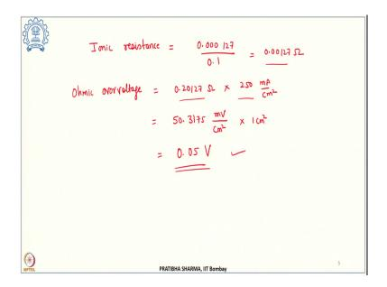
Now, when we substitute that we can get the ionic resistance as 0.000127 ohm and the ohmic over voltage in that case is the sum of the two resistances times the current density, which makes it 50.3175 milli volt per centimeter square or we can also convert it into volts.
