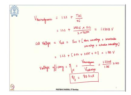
So, using this we can write down the V thermodynamic as the V reversible voltage 1.23 volt plus T $\Delta$ S/nF, that is 1.23 plus temperature is 298.15 kelvin change in the entropy is 0.12 number of electron transfer 2, Faraday's constant is 96500 and on solving this we can get the value of the thermodynamic voltage as 1.23018 volt.
