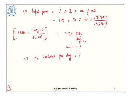
Now, input power we know can be found as the voltage times current times number of cells connected in the electrolyzer. So, number of electrolytic cells connected in series, voltage we have found 1.48, current is 50 amperes, number of cells connected given is 150.
