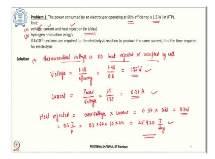
Now, let us look at the 3rd problem statement an electrolyzer, which is having an efficiency of 80 percent and it consumes power of 1.5 watt and that is at room temperature pressure condition. What is required to be found in the problem is what is the corresponding voltage, current and how much is the heat rejected and that is required to be found in joule per day of heat being released?
