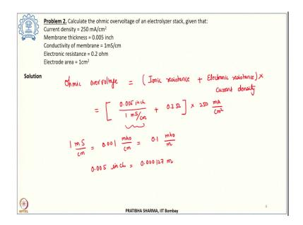
Now, the 2nd problem is it is asked to calculate the ohmic over voltage of an electrolyzer stack.
