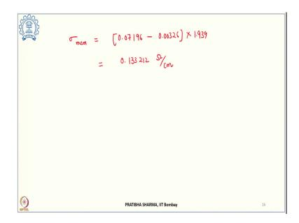
So, the conductivity of the membrane we can write down as this value comes out to be 0.07196 minus second term 0.00326 times the exponential part its value is 1.939. Finally, we get a value of 0.133212 ohm per centimeter. So, that is the conductivity of the membrane that we can find out using the condition that it is under the full humidification condition.
