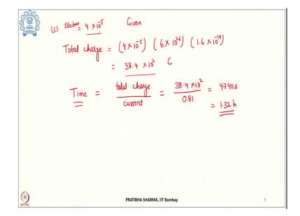
Now, let us look at the part 3 of the problem where it is given that the number of electrons is  $4 \times 10^{-5}$  electrons are required for electrolysis to produce the same current. So, we have to find out the time required for electrolysis in this process and number of electrons is given as  $4 \times 10^{-5}$  this is given in the problem.
