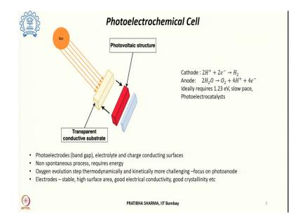
So, a very basic structure, although there are several other layers attached to it is where there is a transparent conducting layer; then there are semiconducting layer and then there could be current collectors or transport layers. So, basically a photoelectrochemical cell just like electrolyse has a basic unit of electrolytic cell; photoelectrochemical cell is the basic unit for the process.
