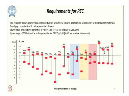
When it comes to photoelectrochemical reaction that occurs at the interface, electrode electrolyte interface. Now, there are several semiconductors which are available which absorb sunlight and then they can produce the charge carriers; but for photoelectrochemical reaction to occur, the band gap is a important measure. So, appropriate selection of semiconductor
