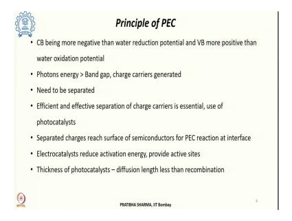
Now, if you look at the basic principle of photoelectrochemical process, we have seen in the earlier figure the requirement is conduction band should be more negative than the water reduction potential and valence band should be more positive than the water oxidation potential. So, what is required is when the sunlight falls on to such material semiconductor material, the required energy of photon should be higher than the band gap.
