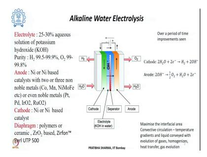
In this class we will see the four different electrolysis technologies. So, the first one is alkaline water electrolys. It is alkaline water electrolysis is a mature technology and it is most widely used global technology for producing hydrogen by means of electrolysis. This is a safe method, this is reliable and it is less expensive compared to the acidic electrolysis, it involves lower cost materials components as compared to the PEM electrolysis.
