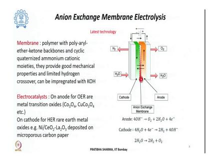
And in the process of this electrolysis, again this is a membrane based method, but it allows anion exchange across the membrane.
