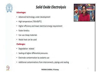
So, the solid oxide electrolysis this is a high temperature electrolysis or a steam electrolysis which takes place at a higher temperature, this is an advanced technology still under development. So, very small capacity demonstrations have been there, it is having a high efficiency. The reason being the required temperature, as we have seen in the earlier classes that total required energy for the electrolysis to take place can come from electrical energy and from thermal energy input.
