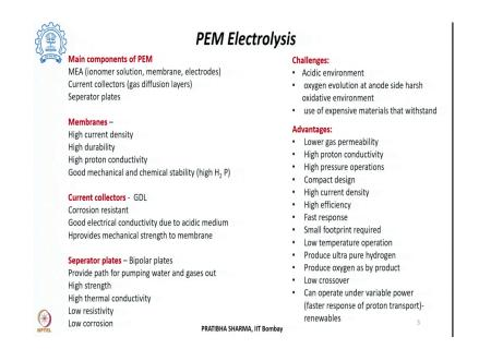
Now, the major components of the PEM electrolysis, Polymer Electrolyte Membrane electrolysis are: this membrane electrode assembly which is the ionomer solution membrane and the two electrodes, the current collectors which is the GDL, Gas Diffusion Layer and the separator plates are the bipolar plates.
