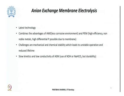
Now, this is the most recent technology, the latest technology and as I mentioned it combines the advantages of both alkaline water electrolysis, the advantage that it has a less corrosive environment.
