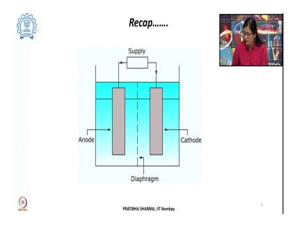
In the last class, we have seen the major components of the electrolytic cell which is the basic unit of an electrolyzer. And, we have seen that it has two electrodes, an electrolyte and a diaphragm separating the two electrodes. Now, these electrode and electrolyte they have an interface depending upon the cell configuration. And, at these interface the various electrochemical reactions take place.
