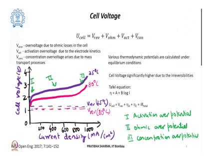
So, under that condition the overall cell voltage is a sum of reversible cell voltage. Another term which is arising because of the ohmic resistance or losses within the cell. Third term which is arising because of the activation over voltage and the last one because of the concentration over voltage. So, the total cell voltage is a sum of all these voltages. First one is the thermodynamic reversible voltage which has a value of 1.23 volt.
