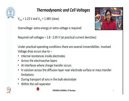
Now, in this voltage the various components of the reacting species are in the gaseous form. So, water is present in the water vapor form. However, the required energy for converting into water vapour, if that also comes from the electrical energy and the process becomes isothermal.
