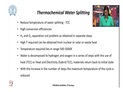
Now, what could be the alternate is thermochemical water splitting. What do we mean by thermochemical water splitting? In thermochemical water splitting there occurs a multiple step reaction, a series of reaction wherein certain chemicals, they undergo a series of processes, they are recycled back to their initial stage. However, the water which is being fed in the reaction that undergoes a splitting to form hydrogen and oxygen, that is what is thermo chemical water splitting.
