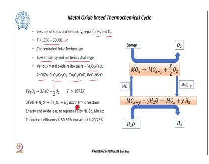
Let us start with the simplest thermochemical cycle which is a two step process involving various metal oxides. The interest in these metal oxide based thermo chemical cycles is because the number of steps involved in the process are only two these are simple. And they produce hydrogen and oxygen separately as such the separation of the two gases is not a problem.
