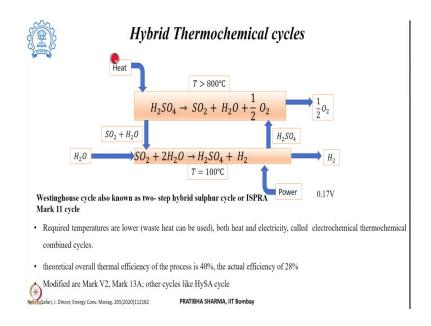
If you look at the hybrid thermal thermochemical cycle as I mentioned that other than the heat input, there could be input in terms of either electrical energy input or it could be photonic also with terms of from light. So, here this is one of the modified sulfuric acid cycle which involves only two steps. The first step where sulfuric acid it decomposes to give SO2, H2O and evolves oxygen, so producing oxygen.
