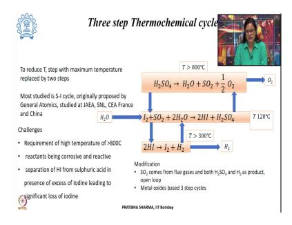
If we look at the three step thermochemical cycle again the reason is that the maximum temperature involved in the two step process was very high. To reduce that this three step thermochemical cycle was identified. There are various such thermochemical cycles and the most studied one is the sulphur iodine cycle.
