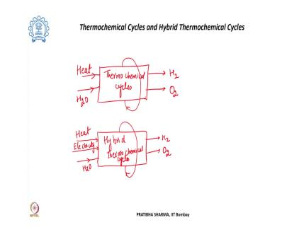
Now, let us understand these thermochemical cycles little better. In the thermochemical cycles, the input which is supplied is heat, it could be either from the nuclear reactor or it could come from the concentrated solar power and water. The materials or chemicals water whatever are being used they get recycled back to their initial stage producing the two products which is hydrogen and oxygen.
