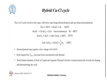
One of such cycle is the hybrid copper chlorine cycle. This involves four steps and these out of these three step one, three and four these are thermochemical steps and the second one is an electrochemical step. So, copper reacting with HCl produce CuCl, this occurs at a temperature of 450 degree centigrade.
