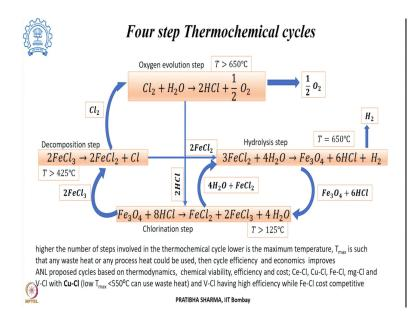
Now, if we include one more step then, so, we know that higher the number of steps involved in the thermochemical cycle lower will be the maximum temperature required in the endothermic step. And if it gets so much lower that if any waste heat or process heat which is available, the industrial waste heat in any of industrial processes, if that could be used for the thermo chemical cycle then the economics as well as the efficiency works very well.
