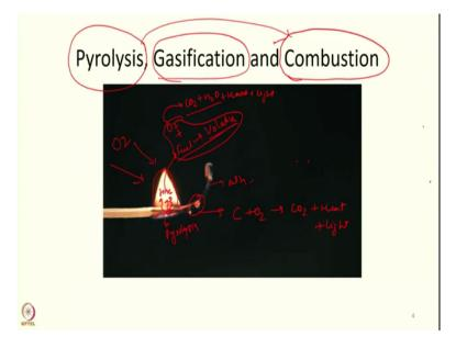
So, when charcoal gets burnt what you get is if your charcoal gets burned finally, you will get ash and then all the combination of all this process is called the combustion. So, here what is happening is, you are doing a pyrolysis here then you are generating fuel that is volatile. And then you are getting oxygen from the surrounding air and this is reacting with oxygen to give you  $CO_2 + H_2O$  + heat + light. So, here we are seeing light also as energy and heat also coming out.
