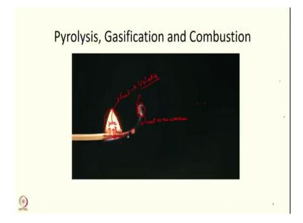
So, lighter compounds when it undergoes it comes out here and this is nothing, but your fuel your higher hydrocarbon is actually coming as fuel and this is called volatile. So, what does this pyrolysis process produce? It produces volatiles and volatiles is nothing but higher hydrocarbon. So, short form for that HHC higher hydrocarbon and oxygenated higher hydrocarbon and plus it also has carbon monoxide, hydrogen, H<sub>2</sub>O, CO<sub>2</sub>.
