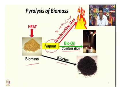
So, pyrolysis, I hope you understood that whenever we are breaking down the biomass by supplying heat pyrolysis happens and in the pyrolysis this biomass is getting converted into something called as vapour. Because it is at high temperature everything you will see it is coming out as a vapour, but if you bring down at the room temperature, then you will see that you will get some as condensate which is technically called as bio oil which is higher
