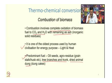
So, thermo chemical conversion, combustion of biomass: so, combustion of biomass is one of the oldest process or the technology that human civilization has invented controlled fire. Control fire was one of the major or one of the I would say the most important finding of the human civilization for the light and heat and keeping the animal away from them. So, this was one of the most significant invention or the discovery by a human civilization.
