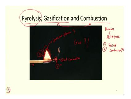
Now, when we talk about the pyrolysis and the gasification, so, these two seems to be a new term how it is different from this combustion. So, this pyrolysis, gasification and combustion so, these are not something which are very much different, but here we will see the combustion involves this pyrolysis and gasification. So, these are quite interlinked. So, I would like to explain it with an example of a this burning match stick.
