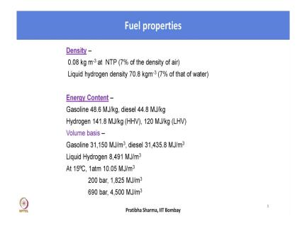
Density of hydrogen is very low. density we know depends on temperature and pressure. For hydrogen at NTP, this is 0.0899 kg/m<sup>3</sup>. When we compare it let us say when we see what is the specific gravity that is defined with respect to a reference material; if it is gaseous then with respect to air if it is liquid then it is with respect to water.
