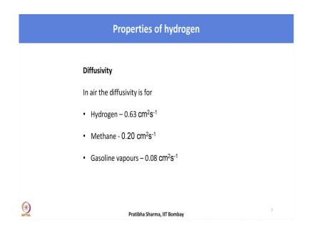
If you look at the fuel properties of hydrogen, hydrogen has a very high diffusivity in air. If we look at these numbers, hydrogen diffusivity is  $0.63 \text{ cm}^2/\text{s}$ . This is 3 times that of natural gas. It is an order of magnitude higher than that of the gasoline vapour.
