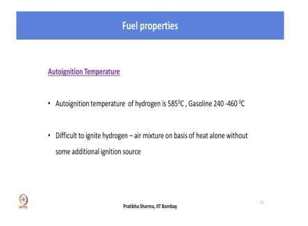
For hydrogen this auto ignition temperature is 585 degree centigrade; however, for gasoline this is lying in the range of 240 to 460 degree centigrade. Now, this higher auto ignition temperature makes it difficult to ignite a hydrogen air mixture, it is difficult to ignite on the basis of heat alone; that means, you require an additional ignition source to initiate combustion. Now, this is an advantage in the sense that in engines where a higher compression ratio is required.
