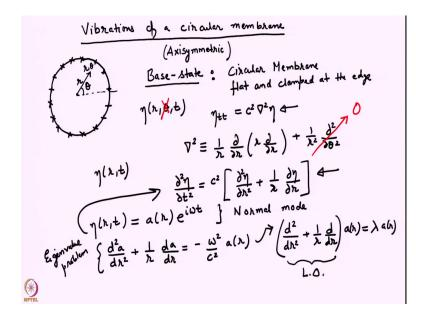
So, our next topic is vibrations of a circular membrane. We had looked at until now we have looked at a rectangular membrane, now we are going to look at a circular membrane. So, this is the center and I am going to use say any point has coordinates r and theta; r is the length of the radius vector up to that point and theta is the angle it makes with the dotted line.
