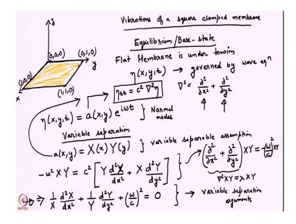
We were looking at Vibrations of a clamped square membrane in two dimensions. It was governed by a linear wave equation a 2D wave equation. We had started with doing normal modes on it and using the kind of coordinate system. It is this was a Cartesian coordinate system and since the membrane was clamped at all ends it allowed us to do variable separation.
