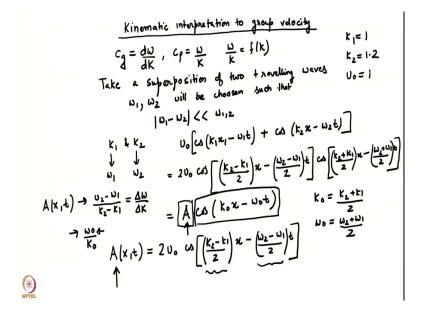
I have chosen the amplitudes to be the same and so, I am just adding them up. We know from the formula of cos a plus cos b that we can write this as now I can write this as some amplitude A into a cos wave which is k 0 x minus omega 0 t. Here k 0 would be k 2 plus k 1
