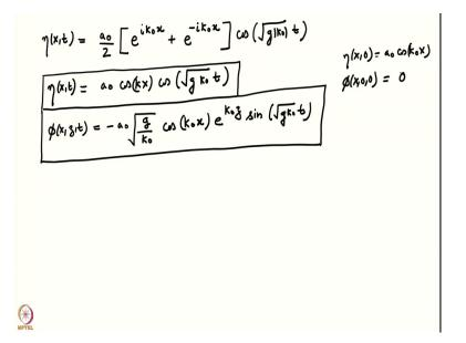
So, you will get that phi of x comma z comma t is equal to minus a 0 square root g by k 0. And because now k 0 is anyway a positive number so, I am; I will just skip writing the mod  $\cos k 0$  of x e to the power k 0 of z sin square root g k 0 into t. So, those are our solutions when the initial condition is a 0 cos k 0 x and phi is 0. You can see that if you put time equal to 0 and z is equal to 0 in these conditions, you will recover the initial conditions.
