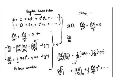
Note the error. The second term in the Taylor series exampsion should be  $\left(\frac{\partial^2 \phi}{\partial z^2}\right)_{z=0} \eta + \dots$  This term contributes only at  $O(\epsilon^2)$
