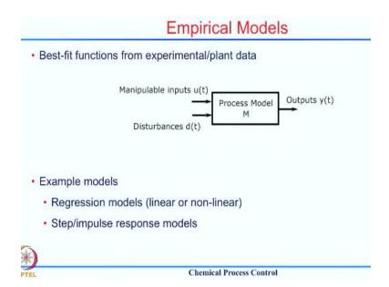
Let us now see what are the other options which are available with us in case the first principle dynamic model has limitations for the process under consideration. In that case, we go with what is known as an empirical model. The empirical model one which will be developed with the help of experiments. As we had seen earlier, a dynamic model is that, which gives you a relationship between inputs and output as a function of time.
