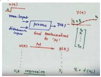
In the early advanced controllers, these type of models were used to capture the response of a process. So the idea is, if there is some input which is given to the process, you can always write it down as a summation of multiple steps and then assuming the process to be linear we can just add the responses corresponding to each of the inputs. Let me explain this phenomenon again.
