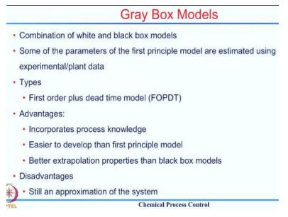
We use some parameters from the first principle model. Typically it is the form of the inputoutput relationship which we get from the fundamental or first principle modeling, and while getting the parameters of the system, we use experiments or empirical data. So in a way it is a combination of the two methodologies and a very commonly used gray box models from a control point of view is known as the first order plus dead time process.
