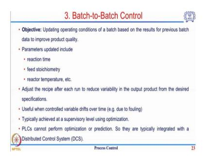
And what typically you would want to update are the time for the reaction, so this is like a batch time. Sometimes there is a stoichiometry which has to be updated. Previous batches if the excess air, let us say was 10% and the conversion was slightly less, the next batch may be operated at, let us say 11% as an excess air. So how do you go from 10 to 11 so that is based on all the previous data which was available?
