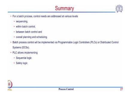
Just to summarize a within batch process control, there are 4 key tasks which you have to do. One is you have to do sequencing in terms of startup and shutdown. Then you have to maintain a certain condition when the batch runs that is within batch control. Then you learn from every batch to batch so all that data would be used in order to improve the next batch which is which becomes part of the batch to batch control.
