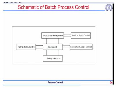
If I want to really schematically show how this looks like, you can see that the equipment which is going to do the batch processing, it has a connection to sequential logic controls. Because that is going to decide how this equipment is going to operate. It also has safety interlocks even though I am showing it differently. It is part of this sequential and logic control. This safety interlocks here I am showing are more like a hardware interlock rather than incorporated within PLCs.
