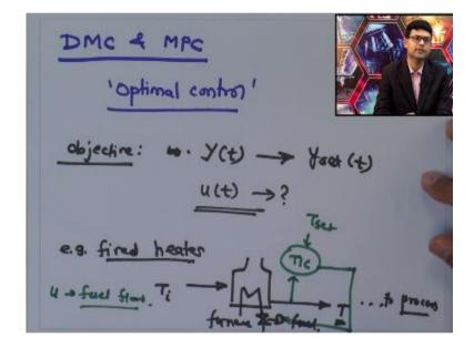
Both these controllers fall under the domain of optimal control and let me first motivate what do we mean by optimal control. So far all the control strategies which we looked at right from a simple PID control, then cascade control or split range control or even for that matter IMC which is Internal Model Control, all the time our objective was to ensure that your output goes to the set value.
