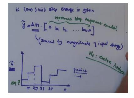
So if non-unit step change is given, then the corresponding y tilde will be  $\Delta m$  times this
