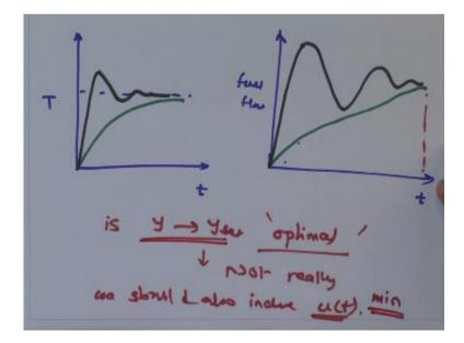
As shown in the figure, 'T' is the set value and here I will show you the fuel flow. One possibility is that you have a very fast controller and it reaches the setpoint value pretty quickly. This is, but the corresponding fuel flow what you require is very large and it varies like this. As against you can also have a different type of a controller which reaches that same temperature and in this case the fuel flow what you will realize is also relatively less compared to the other strategy.
