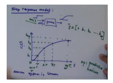
DMC uses what is known as a step response model. In the first few lectures first few weeks of this course, we saw first order dynamics, second order dynamics, and even higher dynamics and how they respond to a step input. This is exactly the same thing. So you give a step input into your process. So you give a step input and you record how your output changes.
