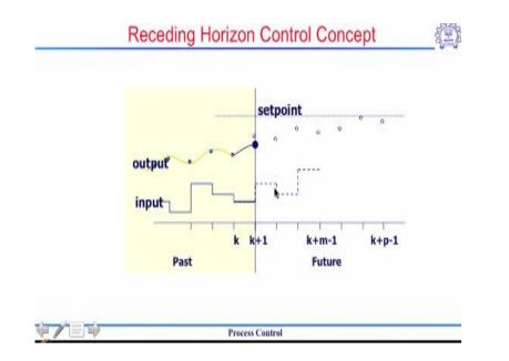
You can see here that this is your process. You had given some sort of inputs and this is how the process is responding and you have a setpoint request for this particular process and here 'k' stands for any time instance. Now what happens in this sort of a controller, you first predict what should be your new future input, so those are shown here. And by using this prediction model you calculate how your output profile looks like.
