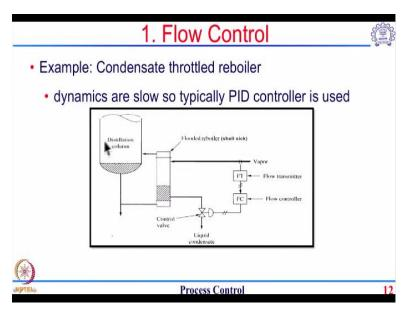
You can see that this is the bottom of the reboiler and we are trying to control the flow of steam which is going to go to the reboiler. This is known as the condensate throttling reboiler, also known as flooded reboiler where the amount of steam which goes into the reboiler is controlled by the amount of heat transfer which is going to happen. So the way this particular reboiler works is that you have this condensate flow.
