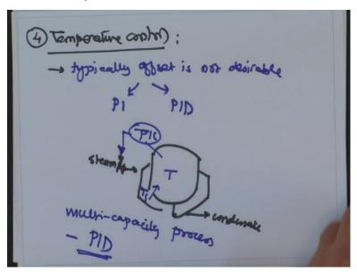
So most of the times temperature is controlled because you want to maintain a certain temperature inside a reactor, which is favoring the kinetics of the desired product. So typically offset is not desirable, so you have two options, one is PI or PID, and again we try to follow similar rules. If the inherent process is fast, you will try to go with a PI controller. If the inherent process is slow or multi-capacity, then we will go with a PID controller.
