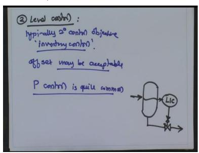
If you look at the example of the flash vessel, you will measure the level and very commonly you would try to control it by changing the outlet flow. So that is how a level controller will be implemented in a process. A lot of times you try to look at what is the outlet flow from that particular vessel and then try to control the level by using that particular flow. Next, we will go to pressure control.
