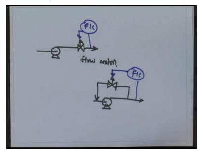
So you have a pump which is going to deliver this flow. So there are two ways in which this flow controller can be implemented. One is simply having a valve at the outlet. So you will measure the flow and then accordingly change the valve opening. If the flow is higher than the set point, you will close the valve opening. So what it does is it changes the resistance across which this pump has to do the work.
