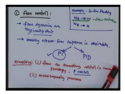
So if you try to recollect the example which we had about the in-line blending. There were 2 options, 2 SISO options. One of those was, controller 1 requires you to control the outlet flow, so this is a flow controller. So if this is the controller which we want to design further then what type of a controller we have to use. So as it turns out, flow dynamics are typically fast, and mostly you want to set a particular flow going to a piece of equipment.
