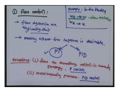
So most of the times flow control will be a PI controller. When it is part of a cascade control and a secondary control objective it will be a P controller. If it is a multicapacity process like a flooded reboiler, then it will be a PID controller. Now let us see how the control loop will look like.
