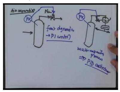
So when you talk about air separation, what you are going to get at the top of this column is nitrogen, which is gas. So the way you can control the pressure inside this column is by simply measuring the pressure and accordingly changing this valve opening. So this is a very fast dynamics, so you can use a PI control. Now this PI controller was possible because we did not have any condenser here and vapor is the product at the top.
