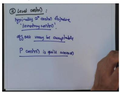
So typically as you recall the example of the flash vessel we implement level controller, not as a primary control objective but typically as a secondary control objective because you want to do some inventory control. You want to maintain a certain inventory of liquid in that particular vessel so that it does not go dry or it does not overflow. So a lot of times offset may be acceptable.
