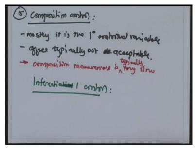
The last type of variable which we commonly want to control, is the composition control and the reason I am saying want to control is a lot of times you will not see a composition controller as a PID controller per se, so mostly it is the primary control objective. The offset is typically not acceptable, so you would typically want to think that it will be a PI or a PID controller and what happens is composition measurement is typically very slow.
