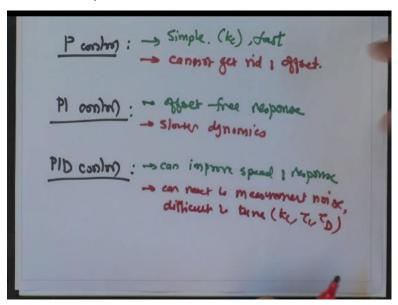
So when we say P control or the proportional control, the main advantage is it's very simple, there is only one variable  $k_c$  which you have to decide. It is often very fast and is based on the current error. On the other hand, when we talk about the limitation, it cannot get rid of offset. That is a major limitation of a P controller.
