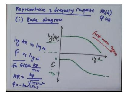
If we go back to a previous figure, what we have seen is at the low frequency we have almost a straight line, horizontal line and at very high frequencies we have a straight line with a slope of -1. Typically for a first-order system the frequency response, the first part of the Bode diagram will look like this and the second part is simply the tan inverse of tau omega. So when omega is=0, we have phase equal to 0.
