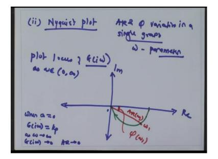
Here instead of computing two figures, we are actually going to compute a single to represent AR and phi in a single graph. So in order to do that what we do is we take frequency as a parameter and then we plot locus of the complex number which was used to obtain this frequency response. So we take G of  $(i\omega)$  as a complex number and we plot this complex number in a complex plane.
