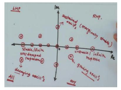
When we have a pole on the real axis, any pole on this real axis in the left half plane with a negative value, what we are going to have is the response will have  $e^{-\lambda t}$  terms which all will decay down to 0. So all these will give you stable response; so stable or finite response, overdamped response. There will be no oscillations in such a case.
