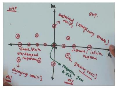
If I say there is a zero at the origin. Then it will give me a response goes to zero. Now for most of the parts, zero would just change the relative contribution which would not be directly predictable. The only case when you can predict the response of zero, so let us try to use a different figure for zero.
