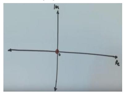
The real axis and the imaginary axis are shown in the above figure. In the figure for any transfer function, we will plot or we will put the poles as well as zeros. So we will start with the poles. Let us say the pole of the system falls at the origin. Let us say if the pole is at the origin. So when the pole of a system or transfer function is at the origin, the denominator of the transfer function will have a term '1/s' or the denominator will have a term 's'.
