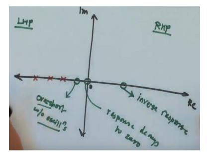
The real part and an imaginary part is shown in the figure. if there was a zero at the origin, the response decays to 0. Now if the zero is on the real negative real axis and it is closer than any of the poles. This zero is on the negative real axis and it is closer than any of the poles to the origin, in that case, you will get overshoot without oscillations obviously. So this was the case when we had overshoot into that first order or second order system.
