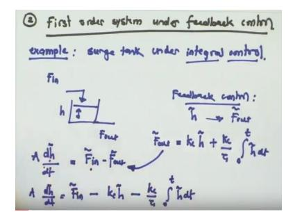
This is our surge tank where we have some feed flow coming in and have the outlet flow. We want to control the level 'h'. Now in terms of the actual dynamics of the system, we had already seen that the height dynamics or the level dynamics of the system in deviation form can be written as
