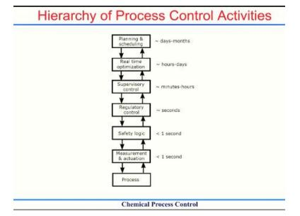
At the bottom layer is your actual process and the first action is the measurement and actuation. This consists of all the instruments which are put into the system either to read value from the process or to take some action on the process. So these are the hardware elements inside the process and they will operate at a very fast rate, let us say at a second level or at the time interval of few seconds.
