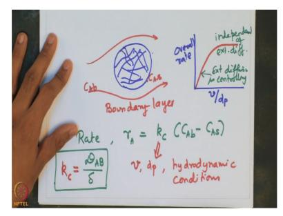
So, let us consider a spherical pellet. And if the species which is in the fluid stream, let us say is actually flowing past to this pellet. Then, there will be a boundary layer which will be present. There will be a boundary layer which will be present around this pellet, because the fluid is actually flowing past this object. Now, suppose the concentration of the species is C A bulk in the bulk fluid. And suppose we assume that the concentration of the species at the surface is given by C A S.
